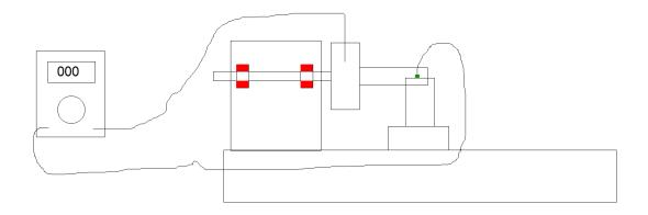
If you connect a common digital ohm meter between the chuck and the cutter, you might read zero ohms. It really isn't zero ohms, just too small for this meter to read. By using a much larger test current and reading the resulting voltage, it is possible to read the tiny resistance.
