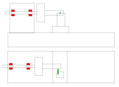
Here you see a simplified drawing of a lathe. The spindle bearings are in red and the cutter is in green. The bearings are held in the headstock which is firmly attached to the ways. The cutter is firmly attached to the tool post which in turn is firmly attached to the apron.
