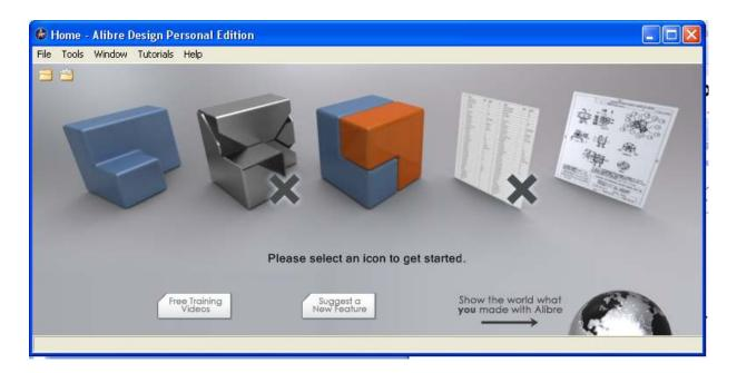
When you want to assemble parts within Alibre, you click on the blue and red cube in the middle of the Home window. A key skill when doing parts assembly is the ability to move parts in 3D space. One way to do this is with the Triad tool.
