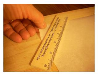
The problem with the rolled paper is it wants to curl back up. This tendency can be reduced by scraping a straight edge against the outside of the curl. I hold the corner with one hand and scrape using the ruler with the other.
