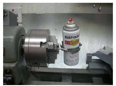
I quickly grew tired of shaking the spray can so used a trick that Rod Grantham showed me – slowly rotate the can when it is not in use.
