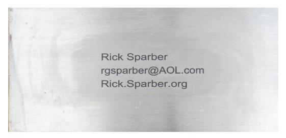
The glue has dried now, and I have wiped the excess from around the text. I did not spray the toner with water.
