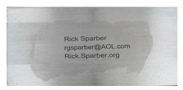
I have now removed the paper. You can see the toner transferred without any breaks. The glue can still be seen in the background. It is still slightly wet. You can take a moist paper towel and wipe up around the text if you like.
