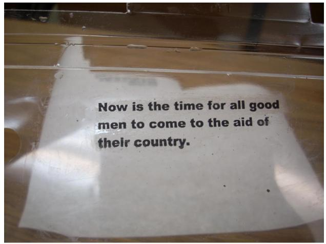
Here is a sample of toner transferred to clear plastic. I'm using Elmer's glue. The white background is just a scrap of parchment paper lying on the table.
