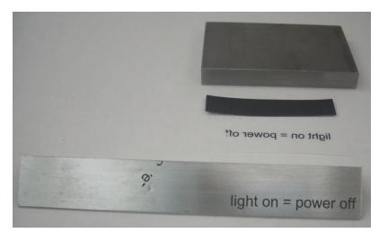
Here is the stack up. At the top is my steel weight. Note that it has a smooth and flat edge to apply an even force to the artwork.
