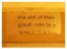
A variation on the above procedure is to print a nonmirror image on the parchment paper. The toner can then be picked up with clear tape. Stick the tape down, and the toner is trapped between the sticky side of the tape and the metal. For light-duty applications, this should work well.
