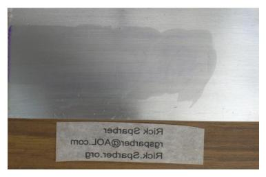
Then I used the card to strike off the surface. This gives me a thin and uniform coating of glue. Note that I draw the card all the way off the surface, so no buildup is left to get in the way.
