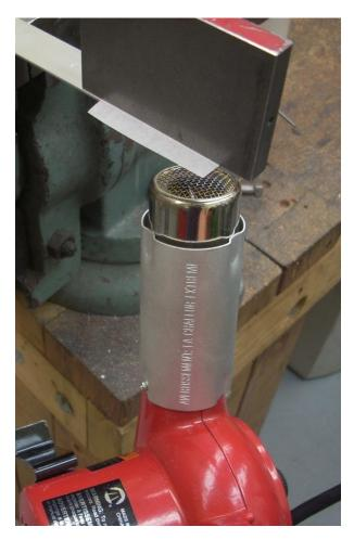
Here is the tricky part – applying heat. I am doing this on the underside because I need to heat the base metal and not the toner. The base metal will fuse to the toner when the temperature is "right." If I just heated the toner, it would run all over that cold metal.
