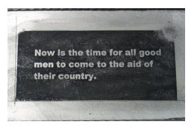
I tried to improve contrast by inverting the image and learned two things. The much larger area of toner tends to cause the parchment paper to jam in the printer. I also found that the large area of toner does not transfer uniformly to the Elmer's glue and metal. I suppose it can be made to work if enough playing around was applied.
