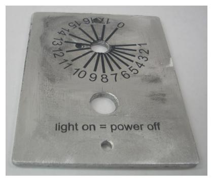
We have finally arrived at my first *useful* project. This is a new cover plate for the speed control on my Gingery drill press. The numbered dial came out nicely, but I did put the text below it on a little crooked. It is all coated with shellac.
