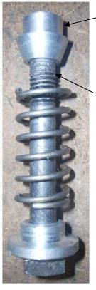
The narrower outside diameter was needed to fit the flat area on the underside of the tailstock.
