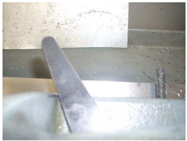
I set up the lock so the tailstock is unlocked with the wrench all the way to the left.
