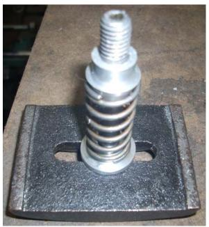
Then I turned the top piece which has a cone to center the spring. The cone was part of the scrap I was using. Otherwise, I would have turned another shoulder.
