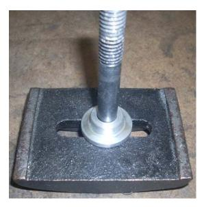
I first turned a shoulder washer. The smaller outside diameter matches this inside diameter of the spring.
