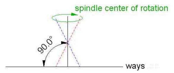
Ideally the center of rotation would be aligned with the Z axis. Rotation should not change its relationship to the ways. If the spindle center of rotation moves as it turns, then we must have this error.
