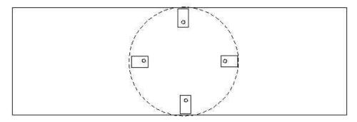
After taking a light cut over the top face of each pad<sup>1</sup>, I would place a dot with a black marker to define the exact location of my reference point. The dot would be as close to the dashed line circle as possible. Then, with the spindle at the center of the circle, I would begin my tramming process.
