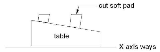
I then mill the tops flat. Even if the head is not trammed, I can get the tops of these pads arbitrarily flat by making each pass over the surface close to the last one. In the above example, we are only dealing in two dimensions so a single pass is sufficient. I now have the top face of each soft pad parallel to the X axis ways. If I now tram the head by referencing these pads, I will have my spindle axis perpendicular to the X axis.
