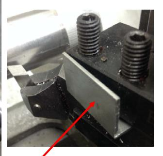
A closer look reveals a piece of thin aluminum angle stock<sup>1</sup> which is captured between the front two set screws and the cutter.
