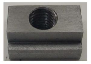
If you have a machine with T-slots, then owning T-nuts is a must. The T-nut slides into the T-slot and provides an anchor port for clamping things to the table. It is an extremely versatile system that has been around for a long time.
