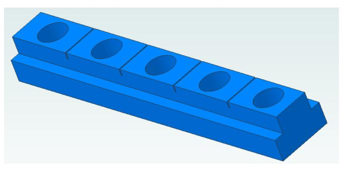
I could drill the hole in one pass but it would be rough on the drill and on my mill. Instead I "step drill", using a 1/4" drill and follow with the 27/64".
