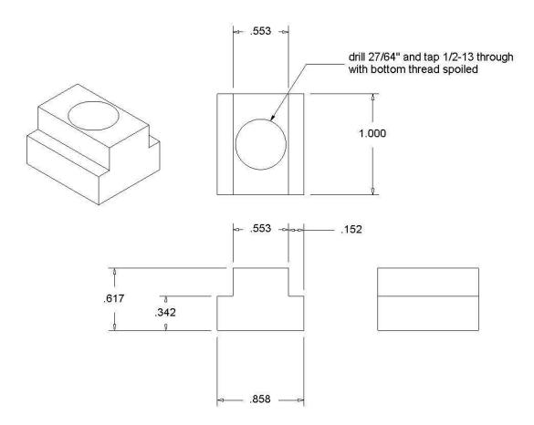
The important bit is that all dimensions and shapes are clear and accurate. Now would be a good time to take the dimensions off of the plans and verify them on the T-slot.
