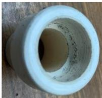
I bored out the end for a tight fit to the pipe that broke off.
