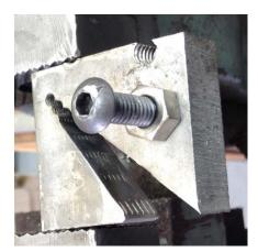
The nut was tightened with an 8" wrench. I then put my torque wrench on the button head screw and it started to rotate with a torque of less than 10 inchpounds. The nut did not move.
