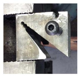
You can see that none of the clamping force is applied to the bolt. The bolt is a high quality button head screw. I was able to develop 75 inch-pounds of torque before the bolt started to turn. It did not fail.
