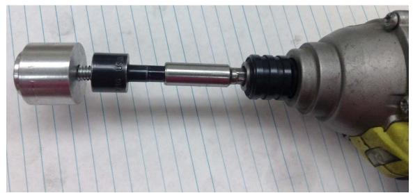
If you thread a ¼-20 bolt into a blind hole tapped ¼-20, it will present an increasing resistance as it reaches the shallower thread. You can tighten down until the bolt starts to fail, yet will easily come right out when you unscrew it.
