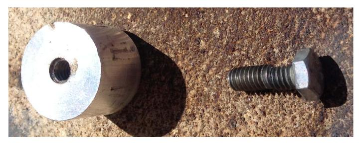
Although I thought it was permanent, by applying the torch to the knob for 20 seconds I was able to easily unscrew the failed bolt.
