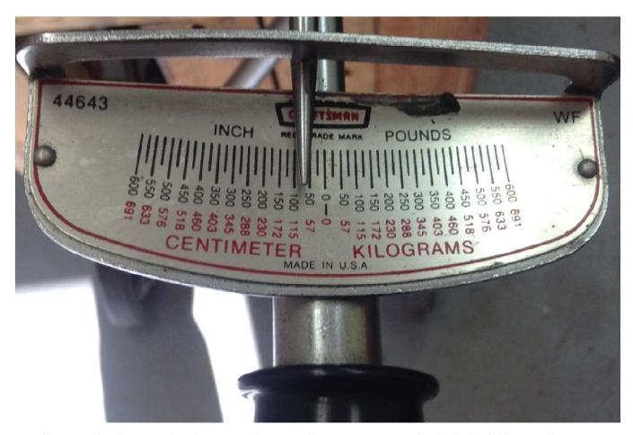
At about 75 inch-pounds, the wrench started to turn. It was the bolt in failure. The bolt never turned in the knob.
