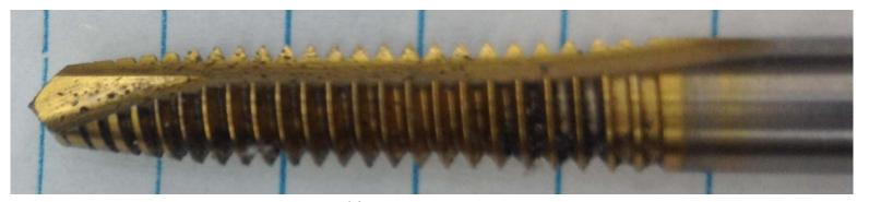
Take a close look at a typical ¼-20 spiral tap. The thread starts out very shallow near the point and tapers up to full depth before you are in ¼". If you wanted the thread to be usable through the entire hole, the tap would have to extend about ¼" out the other side. If the hole was blind, a bottoming tap would get you closer but a few threads would still be too shallow to accept the bolt.
