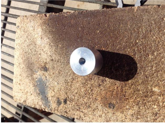
One answer is to heat the knob with a torch. This will cause the threaded hole to expand. I used a MAPP™ gas torch and shot the flame directly into the hole for 20 seconds.
