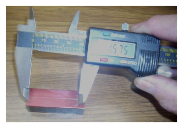
Measuring from the trued up end, I scribed a line at 0.225'' which is my 0.1'' plus the radius of the hole for the head of my screw (0.1'' + 0.125''). The second hole is 1.575'' from that same edge. Here you see my caliper set to this value. I will then put one blade against the trued up end and mark my line across the center line.
