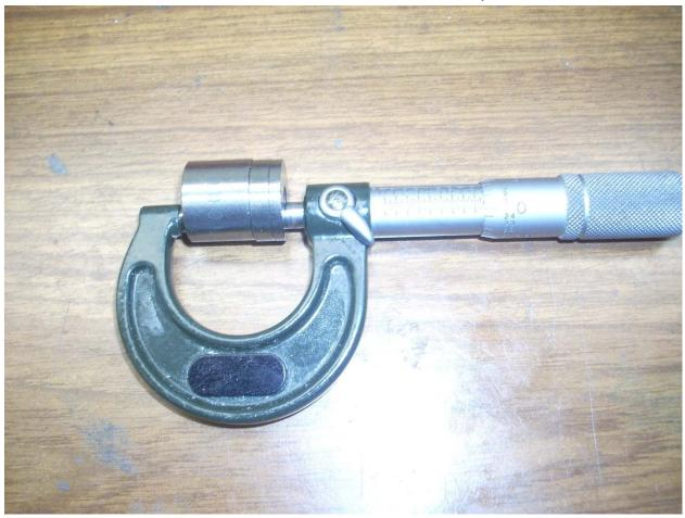
Once I am within 0.01"r of the finished bore, I switch to my micrometer.
