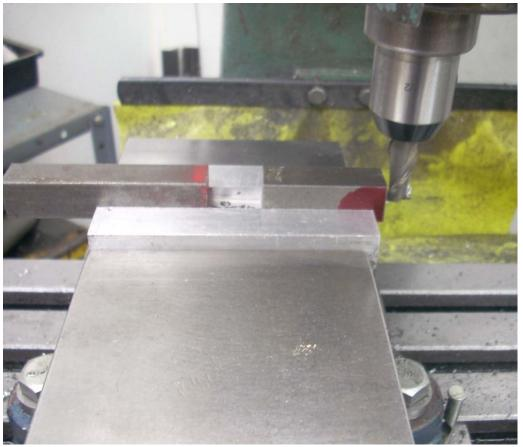
You are looking at my mill vise which has steps cut into the top edges to hold the part. On the right is our clamp bar with the sawn face next to my end mill. On the left is the rest of the bar. It is being used as a spacer so the movable jaw of my vise doesn't twist.
