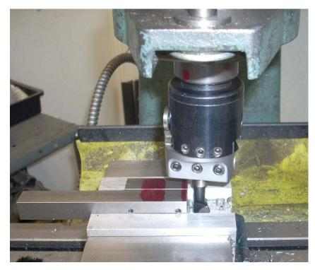
It is time to move the head on my RF-30 mill/drill. Its height must be such that I can fit in my boring head as well as my 5/8" drill. Both are trial fit before the head is locked to the column.
