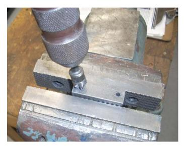
I then use a countersink mounted in a brace and bit to deburr both ends of each hole.
