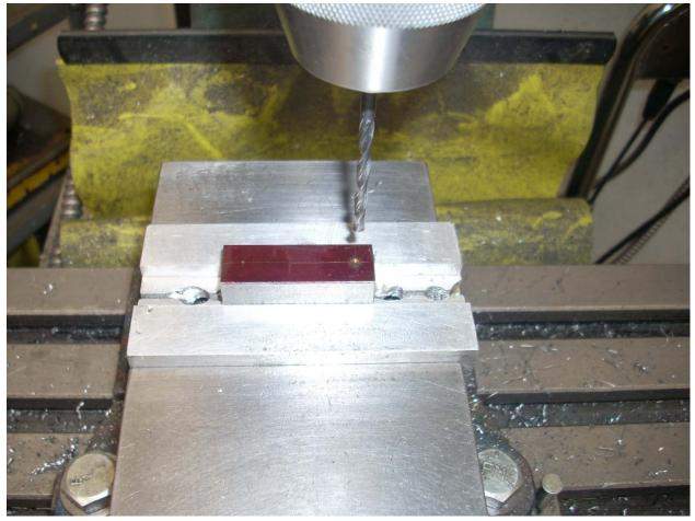
The clamp block is placed back in my vise. The fasteners have a 10-24 thread which means I need a #25 tap hole and a #9 clearance hole. Now, I really don't care if these holes are precisely located but I do want the holes in the clamp block to match up with the holes in the support bar. I have chosen a procedure to insure that this happens.
