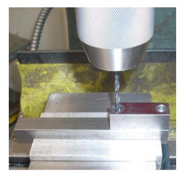
Here you see the two bars lined up. I then raise the drill, remove the clamp bar, and drill through the support bar.
