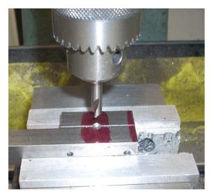
I'm now using my ¼" centering drill to provide a cone shaped hole for my first drill.
