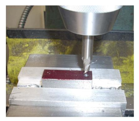
I am using a 2 flute end mill here which can be used to drill holes because it is able to "center cut". A 4 flute end mill cannot typically center cut so would not be a good choice for drilling holes. But since I already have the hole made with the #25 drill, I could use a 4 flute end mill here if I wanted. I touch down the cutter without the mill running, set my zero, then raise it up, turn on the mill, and lower the cutter  $\frac{1}{4}$ " below the surface.
