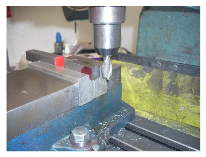
The end of the clamp bar has now been trued up via side milling. I only took off around 0.01". This is just enough to get the end square. I will not square up the other end now but wait until final assembly. In this way I will be able to cut both support and clamp bar at the same time to make them perfectly line up without having to precision measure them.
