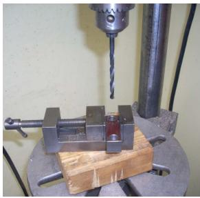
I can now open out the first hole in the clamp block to my clearance diameter. I don't want to disturb my mill so will use my Gingery drill press and homemade vise for the task.
