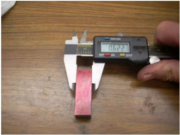
With the clamp block deburred, I first use my red dye on the surface. I then lay out my lines that will locate my two screw holes. To start, I measure the actual width of the block. Minor surprise here. I thought I was using ½" bar but it is actually closer to 5/8". It doesn't really change anything.
