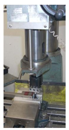
Although not ideal from a support standpoint, my boring head will be cutting with the quill all the way down.
