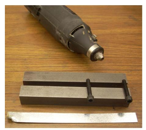
steel (CRS) attached together with a pair of socket head screws. I will call the long bar the support and short bar the clamp.
