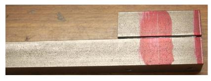
With it all assembled, I then used my Dykem again. I have marked the centerline of the hole to be bored plus how much to clean up at the right
