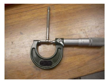
A light touch on the mic is essential. It should go without saying that all surfaces must be free of swarf or grit. This includes the bore.
