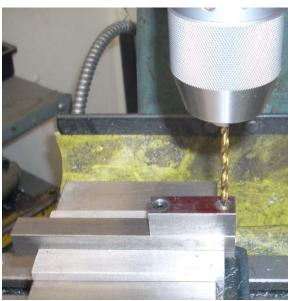
I can now use one of the screws to bolt the clamp block to the support bar. I then put in my #25 drill and move the X axis until it freely goes into the second hole. The clamp block is then swung out of the way and the second hole is made in the support block. I should have started the hole with a centering drill but cheated and just used the #25 drill. It worked OK but is not the best practice. The drill did wander a little before starting to cut.
