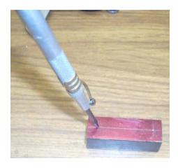
These scribe lines are a little hard to see so I am using a mark out spring loaded punch at each intersection.
