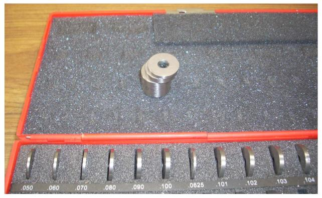
The first step is to have an accurate distance of 0.8750". I own a set of spacer blocks that are good to within +/- 0.0001".
