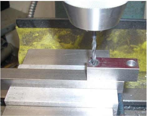
The support bar is put back in my vise. With my #25 drill in the chuck, I lower it part way down through the clamp bar. The mill table's Y axis is moved until the two bars are aligned front to back. I then move the X axis until the ends line up.
