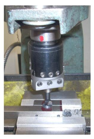
The boring bar is set to just touch the inside of the drilled hole. I want to bore a hole 7/8" in diameter which is 0.8750". This hole does not have to be very precise but I need the practice so will do the best I can. This means being able to know when I'm at the correct diameter.
