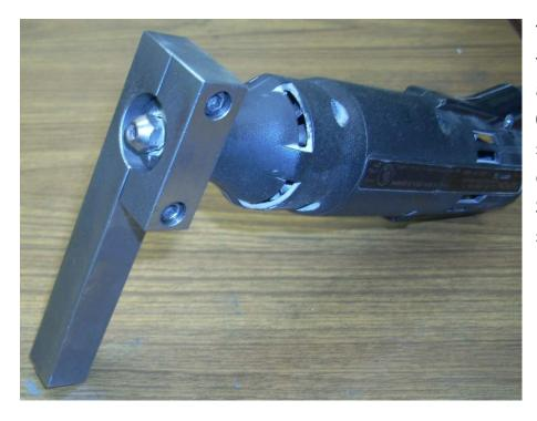
You might be able to see the approximately 0.014" gap between support bar and clamp bar. The High Speed Rotary Tool is securely held.
