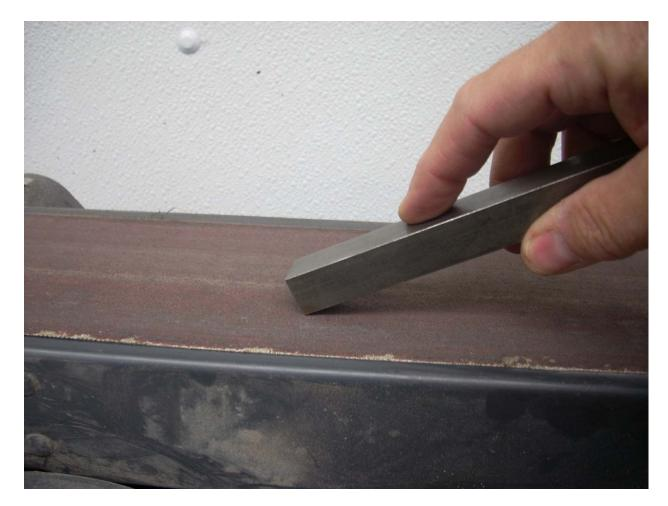
After milling the end, I deburred the edges on my belt sander. It is amazing how well these machines remove metal.
