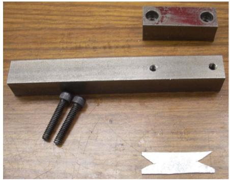
In order to get a good clamping action on the nose of the High Speed Rotary Tool, I will put a strip of that sheet metal between the clamp block and support bar. I have notched it out so it will be captured by the screws. The bored hole will then have a gap the thickness of this
