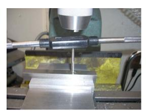
The tap goes in far enough to be secured in the hole. A tap handle can then be attached to finish the job.
