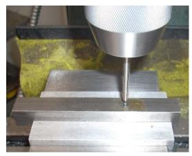
put plenty of cutting oil in the hole, and bring the mill up to speed. Then, with the tap just above the hole, I cut power and feed down. These spiral point taps are designed to just feed in and not be periodically turned backwards to break the chip as is necessary with a hand tap.
