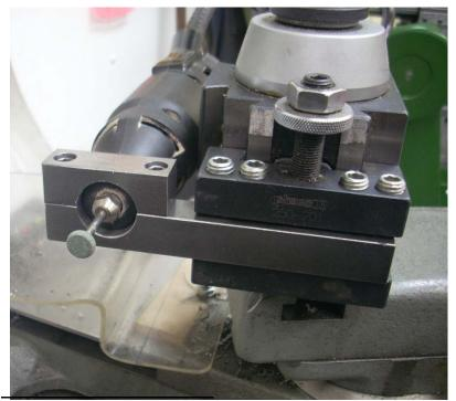
A High Speed Rotary Tool is downright handy at times. And it can be made even more useful if solidly supported in a lathe tool post. Recently I heard this called a "live cutter".
