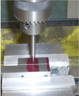
I'm using a pointed length of ¼" rod, called a spud, in my drill chuck. It makes it easy to align the spindle with the center of the hole to be bored out. The X and Y axes are then locked.
