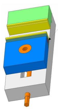
I have removed the sheet metal cover over the pusher block and movable jaw. The cover keeps the (red) half rod in place plus keeps swarf out of the gap between the two blocks.
