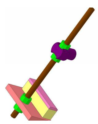
This view gives a better idea of how the bottom nut works. The two Acme nuts are separated by 0.8". The thread is a  $\frac{1}{2}$ -10. This means that I should have 8 threads inside the bottom nut and the Acme nuts should be snug on the pockets of the bottom nut.
