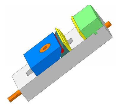
The half rod is easier to see in this side view. I have a 0.1" gap between pusher block and movable jaw. I could cut the half round deeper in the movable jaw and cut the half rod so more than half of it is left. That might make machining it a little easier.
