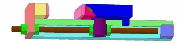
I have removed one side of the base and you can see the bottom nut and the antirotation stop attached to the pusher block. The spacer block can be seen on the back.
