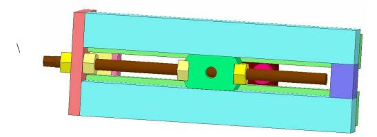
This bottom view shows the new bottom nut, suggest by JRW of valleymetal. It has a much larger contact area with the underside of the ways. This should spread the top nut clamping force over a wider area.
