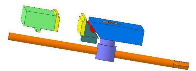
With the base removed, you can see how the leadscrew nut relates to the pusher block. The step in the nut presses on a ledge inside the base to prevent the pusher block from rising up too much. The nut almost touches the top threaded washer. In this way I can adjust the amount the pusher block can rise yet not bind on the base.
