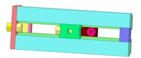
Here you can see the limited rotation stop (in red) fixed to the movable jaw. I have changed from a square block which would need two screws to prevent rotation to a round block which only needs one screw.
