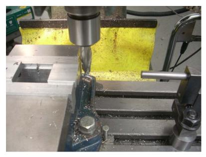
Once clamped, the 1-2-3 blocks are removed. I then took a light cut to define my reference surface. Then I fed in another 0.01" to be sure I always cut the full width.
