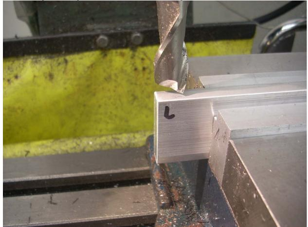
I then clamped the bar in my vise and brought my 5/8" two flute end mill down on the right end. My DRO was zeroed. Moving over to the left end, I brought my end mill down to just touch the surface. I read a rise of 0.0035". This tells me my part is squarely bedded in the vise.
