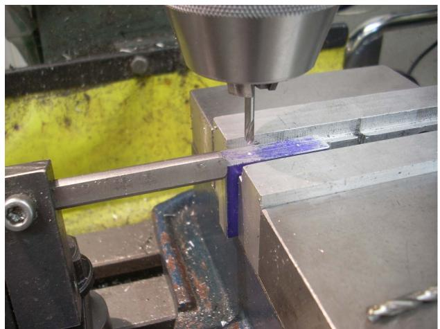
Cutting the square holes was certainly demanding. I got to relax with the next step. Using my 1/8" diameter spot drill, I drilled the location of the two end holes which will later be tapped.
