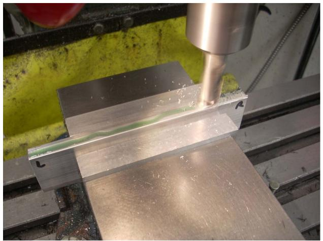
I then took a light cut and zeroed my Z axis. This establishes my initial reference surface. I then set my caliper to zero with it pressed against my stack of spacer blocks. The caliper was then used to measure how much more I must mill from the edge to get my finished width. When done, the bar was removed from the vise, deburred, and cleaned.
