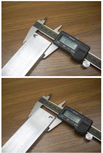
Within the repeatability of the caliper, I hit my number. Now, it might sound like I was being a bit "anal" setting the end mill height, but I used this height for milling all of my bars to width. So some care at set up gave me a good payback later. Even a small error in set up should keep me within my spec of  $\pm 0.005$ ".
