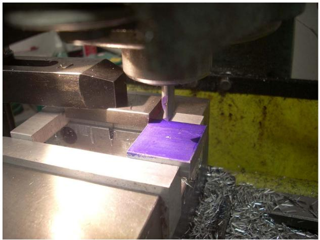
My DRO's X axis was set to zero while cutting the right edge. I used my Electronic Edge Finder to set the Y axis zero. From there I was able to dial in the center of my square hole. This became my new (0,0) position. The plan was to knock a 1/2" diameter hole and then use my 1/4" end mill to square it up.
