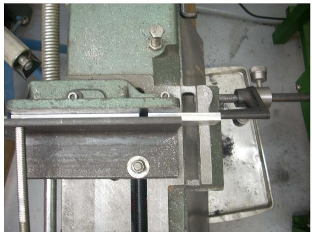
The next step was to cut each 6" bar into 1.3" long blocks. This will give me 0.05" of material to square it up on my mill. The first block was carefully set in my bandsaw vise and the stop set.
