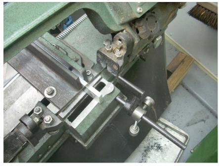
Before starting the saw, I moved the stop out of the way. Failure to do this can cause the part to twist and jam as the blade finishes its cut.
