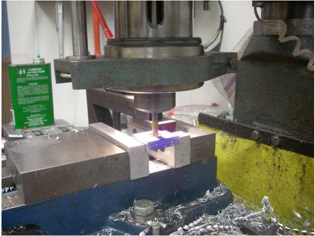
The final milling step for the square hole requires my 1/4" end mill. I swapped out my 1/2" collet for my 1/4" collet and locked in this end mill. Because I used collets for all of these operations, I didn't have to raise or lower my mill head which would have required me to reestablish my zero.
