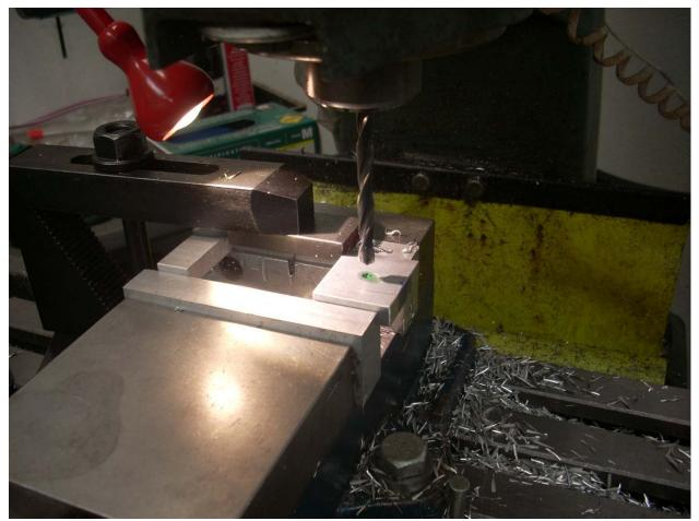
The next step was to install my 1/4" drill and put a tiny drop of cutting fluid in the cone shaped hole left by the spot drill. I am through drilling now so it is easy to just feel for the drop in resistance as I broke though the bottom of the part. Again, all blocks were drilled. I didn't bother to deburr because the reference surfaces held in my vise were still smooth and clean.
