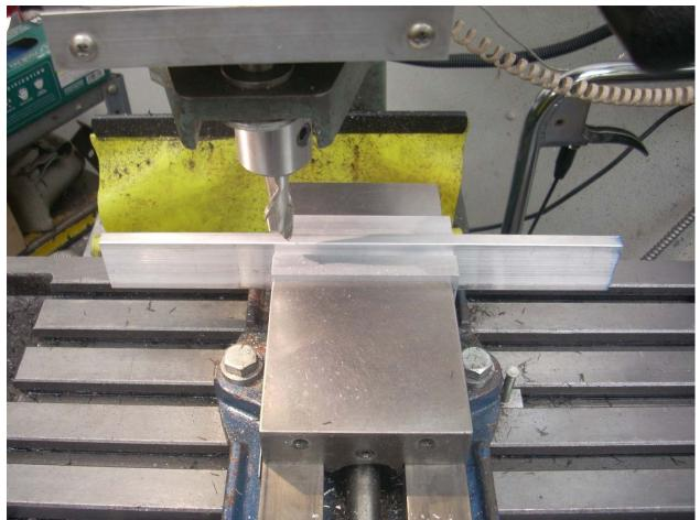
The parts must be 3/8" thick and  $1.491 \pm 0.005$ " wide. I was able to find 3/8" x 1.5" x 12" bar stock. My vise is 4" wide. So if I just clamped the bar stock in the vise to mill the width, there would be excessive overhang. So instead I cut each bar in half.
