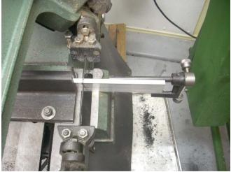
Most of the time in my shop, I am making "one-offs" that are cut to fit with other parts. But with this part, I must hit an absolute number. To do this, I used my spacer blocks to define a width of  $1.491 \pm 0.0004$ ". This is a worst case error given that each block has an error of  $\pm 0.0001$ ".
