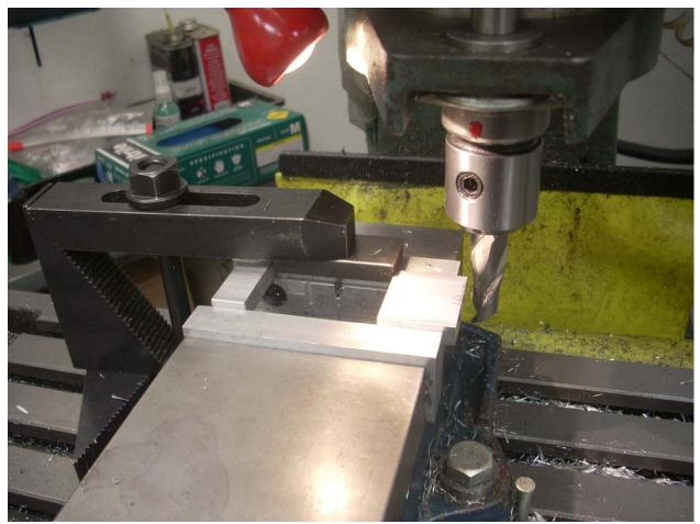
Next I set up a fence on the left edge. This edge was the one that I squared up in the last step. I took a light cut, measured the part's width, and adjusted the X axis to cut the finished dimension. The first part was checked and a fine adjustment was made. The DRO's X axis was set to zero with allowance for the radius of the tool. Then I was able to cut all of the blocks with no further changes to the mill. I did do spot checks of the cut parts to be sure nothing shifted.
