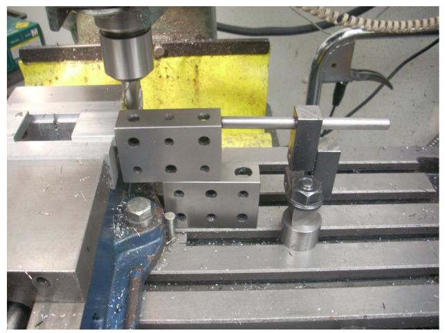
The next step was to square up one edge of each block. I could have put up a stop that touched the left edge of the block but did not trust that my saw cuts were all that square. So instead I set up a stop on the edge about to be cut. The two 1-2-3 blocks let me position the work piece.
