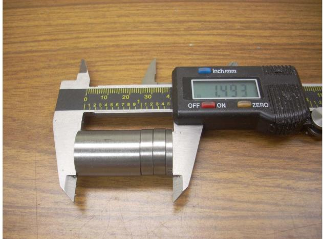
Note that my caliper reads 1.493" so clearly the caliper is not as accurate as my stack of blocks. Furthermore, the caliper has a display repeatability of  $\pm 0.0005$ ". There is also error associated with my skill to hold the caliper square to the pieces. By repeated measurements, I can minimize this skill related error.
