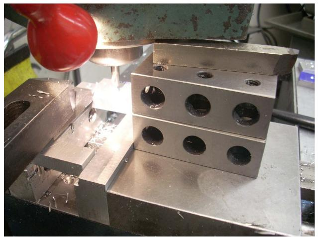
Drilling the cone shaped hole with the spot drill is not a critical step but that doesn't mean that I could not benefit from using a stop. I put down my two 1-2-3 blocks with a cutter on top. In this way I just drop in the part, pull down until the bottom of the spindle bearing housing hits the stop, and back the cutter away. Quick yet repeatable.
