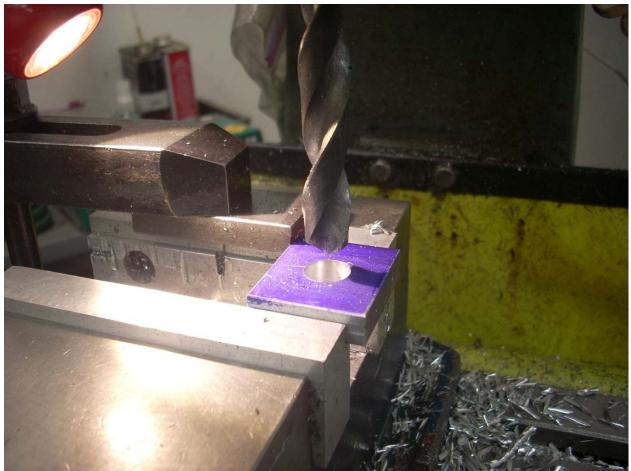
With the 1/4" R8 collet replaced by my 1/2" collet, I mounted my 1/2" drill. All blocks were drilled through.
