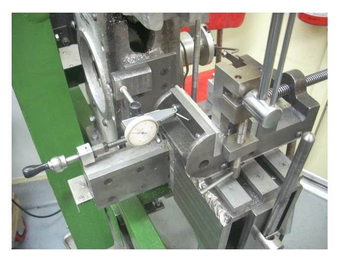
My next test includes the vertical and horizontal ways. I have already determined that the horizontal ways are snug so I am mostly looking at the vertical ways. I applied + and - 150 inch pounds and saw 0.0135" of movement. Clearly something is loose here. I tightened the vertical ways until they locked yet still saw the same flexure. OK, then what else could it be? I've never liked this cheap cast iron vise. Maybe it is the problem.
