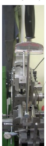
The "magic" combination here is a beam torque wrench and a Dial Test Indicator.
