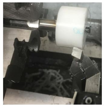
Then I turned the OD using light cuts. I chose a diameter of 1.200" giving me an offset of 0.600".
