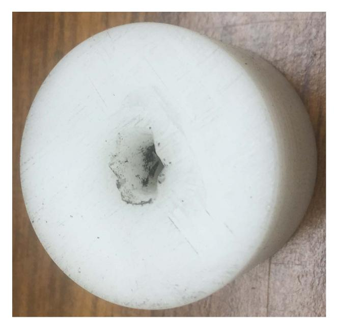
You can see the complex shaped hole formed by the hot end mill melting the acetyl. Since the plastic shrunk a little as it cooled, this is a nice, sliding fit.
