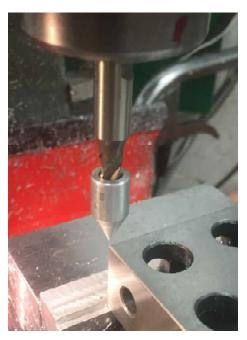
If I am using a 3 or 4 flute ¼" end mill, I can slide on this aluminum sleeve.
