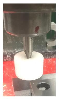
My solution for two flute end mills is to mold a puck of Acetyl onto an end mill and then true it up on the lathe. This puck screws onto the end mill when needed.
