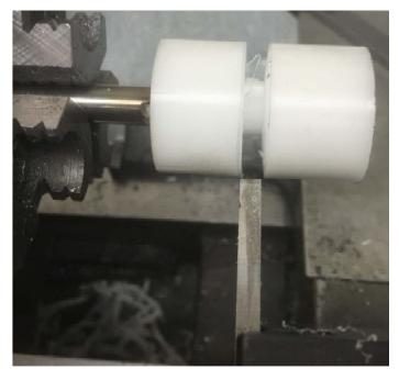
The plastic should be tight on the end mill. Remove the end mill from the tailstock chuck and mount it in the 3 jaw chuck. Part off *beyond* the end of the end mill.
