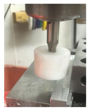
Here I am preparing to touch down for my Y axis. It is easy to sight between the puck and the reference surface and watch the gap go to zero. Since the plastic deforms, overshooting touchdown by a few thou is harmless.
