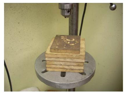
I'm sure we all have a stack of random scraps of wood that we use to quickly change the height of our work surface on our drill press. About 6 months ago I replaced that mess with a pile of identical squares of <sup>1</sup>/<sub>2</sub>" MDF. After drilling countless holes, I have come to appreciate this minor change. The surface does not rock, can be raised in <sup>1</sup>/<sub>2</sub>" steps, and
