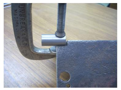
The resulting V accurately holds a short piece of ½" rod as shown above. The C clamp is needed until I can weld the rod in place.
