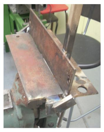
Here is the finished brake. A small block has been welded to the vertical part of the fixed table. The block is held in my bench vise so there is no need to make a support for it.
