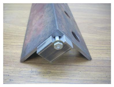
A length of threaded rod was used to hold these blocks in place until they could be welded. Note that the ends of the angle have been machined true. This is necessary in order to prevent binding of the hinge.
