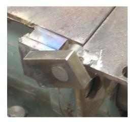
Here is a close up of the second hinge. I thought I had figured the width correctly but discovered that an additional ¼" of width was needed on the fixed part of the table. Not a problem – just tacked on a scrap of steel.
