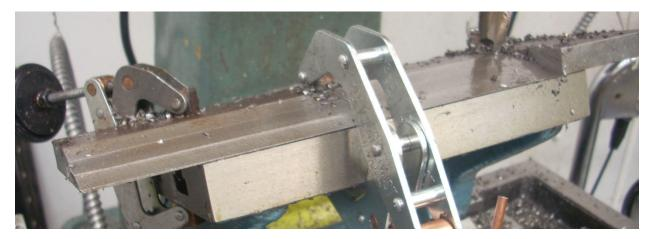
front clamp as needed to let the cutter pass. I was unable to mill all the way to the right end due to limitations in my X axis. I could have removed my vise and had room to shift the assembly over but that seemed like a lot of work.
