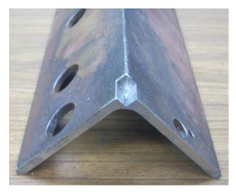
Alignment of the hinge was accomplished by putting the movable part of the table in my mill vise and machining a notch in each end that was 0.250" wide and 0.250" deep.
