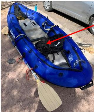
Without the skeg, when I stop paddling, my kayak rotates around where I sit and ends up pointing in the opposite direction. I figure that the further the skeg is from this pivot point, the more effective it will be in keeping me pointing correctly.
