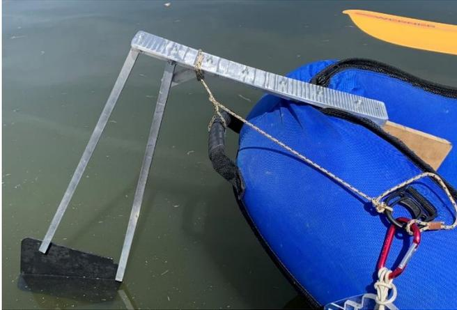
The paracord connecting the diagonal brace to a ring on the gunnel is consistent with the general rule related to kayaks: all items must be attached because we will capsize eventually.
