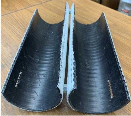
My second iteration involved cutting the pipes both axially and radially. At half the length and by being open, I figured the drag should be reduced. But as I looked at that corrugation, I knew it was still a problem. In fact, I never even tested this version. But it did get me thinking.
