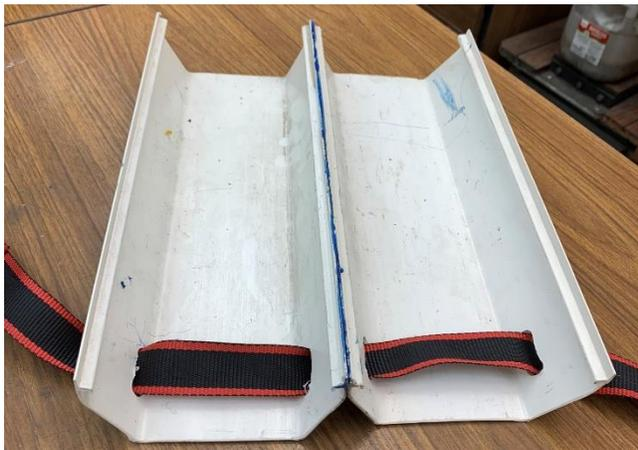
I had some PVC rain gutter. It was thin and smooth. I cut off two lengths about 12 inches long and cut 1 inch wide slots for the strap. Then I used PVC cement to weld them together. It was necessary to clamp the surfaces together about every inch to be sure the surfaces were in full contact.
