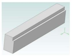
I usually align my vise jaw mounted softjaws by taking a light clean up cut with an end mill. I mill across the horizontal and vertical surfaces at the
