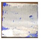
I used a scraper to remove these high spots. I'm not trying to scrape the surface true, just expose the area with ripple in hopes of the Hi-Spot making them easier to see. I've got a few new high spots to scrape off.
