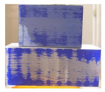
All of the previous tests were done with 6061 aluminum. The top sample here is CRS. It is sitting on the previous sample for comparison. The ripple is still evident but the period is longer on the steel than on the aluminum. This implies to me that I am looking at a resonance condition.
