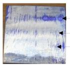
Now I'm seeing the central area. I believe I am seeing three rows of fine lines. Each row is the crest of a ripple. Yet riding on each ripple are these perpendicular ridges that must be formed by the cutter.
