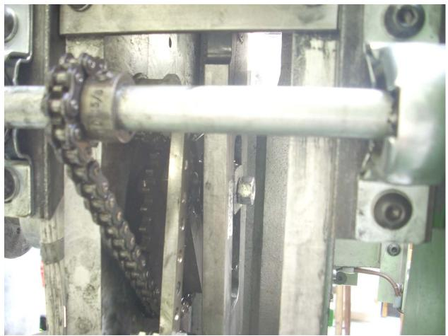
The tensioner wheel can barely be seen above the jack shaft. It is supported by the bar with the equally spaced holes in it. At the bottom of this bar is a bolt that connects to a spring. The spring is connected to the back, rear cross bolt. This arrangement was quick to try but may be replaced by a more ridged wheel support.
