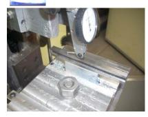
"Rexarino" suggested placing a parallel down on the cut surface to look for ripple. I did not see any regular vertical motion but even a slight pressure on the front or back end of the ram causes a change in the DTI's needle of around 0.001".
