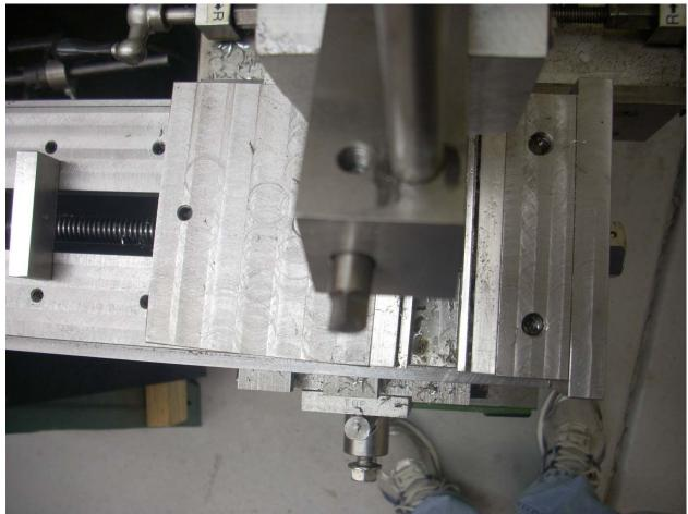
As an aside, here is the cutter mounted in the clapper block. It was ground from  $\frac{1}{4}''$  HSS. Yup, those are my feet...
