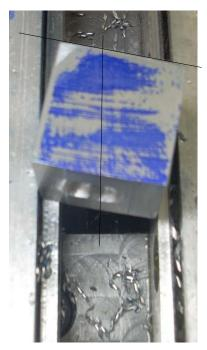
As per John Martin's suggestion, I turned the block so the initial contact of the cutter was not perpendicular to the motion of the ram. It seems that this reduced the ripple. It does appear to me that the ripple is still perpendicular to the ram's motion and not the edge of the block.
