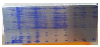
In this sample of aluminum, the block was moved closer to the column. The wider strip on top was cut normally. The narrower strip on the bottom was cut with a heavy weight resting on the head. It cut deeper but what I find more interesting is that the ripples are in the
