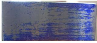
This sample was cut after I added a chain tensioner which will be discussed later. It is hard to see with the Hi-Spot, but when I catch the light just right on the clean surface, I still see the ripple. But now, I can't feel it. When I run my DTI across the surface, I see a
