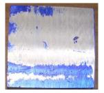
After cutting the surface and deburring the edges, I put a thin coat of Hi-Spot on my surface place and then pressed the cut surface down on it. You can see that the area where the cutter initially hits the block is higher than most of the rest of the surface. That alone is interesting since I always thought it looked like it was lower.
