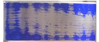
This sample is 1" wide. The shaper is set to minimum speed and minimum cross feed. The cutter is a sheer set at 45°.
