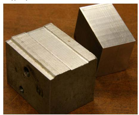
It is hard to see the difference in this picture, but the tilted block was cut on my new vise and has a better surface finish. The other block was held in my old, weak vise which permitted movement during the cut.
