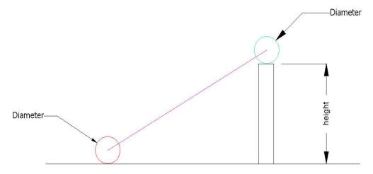
Look what happens if I put one of the cylinders on a block of known height. The line between centers will now be at an angle with respect to the horizontal.
