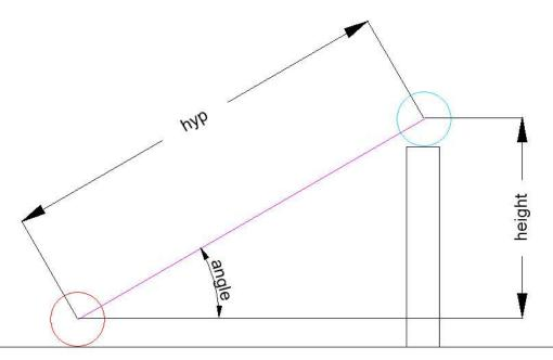
Here is where having the two cylinders with the exact same radius comes in handy. The lower end of the sloped line is one radius above my flat surface. The upper end is a one radius above the top of our block. So if I draw a horizontal line from the lower cylinder's center over to the block, I will be one radius above the flat surface which is supporting my block.
