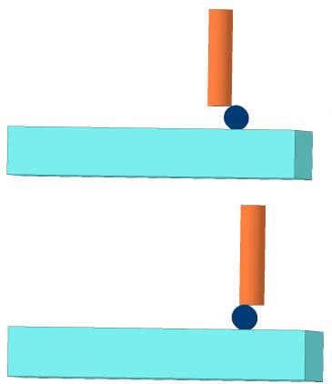
Next the end mill is jogged *upward* as the dowel pin remains in contact with the bottom edge. You can see how, as we raise the end mill, the dowel pin moves under it.
