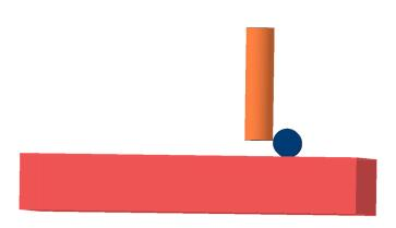
The solution is to use a precision round dowel pin. The pin lays down on the reference surface. It is rolled until it touches the end mill which is less than its diameter from the reference surface.
