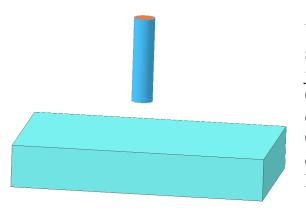
When establishing an end mill above a reference surface using a CNC machine, the operator must jog the cutter down in discrete steps. Even at 0.0001" per step, there comes a point where the cutter crashes. The crash might be only 0.00005", but that can be enough to crack the cutting edge given that the reference surface is hardened
