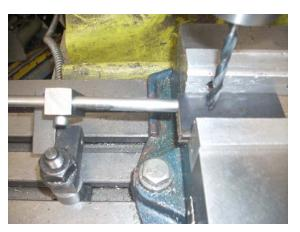
After cutting this strap, I needed to drill a hole on the centerline and 3/4" from each end. This is another good place for a stop. This stop is homemade and bolts into a T-slot. I am holding the strap in my vise so the fixed jaw is another stop. And finally, I put down a strip of Medium Density Fiberboard that is slightly narrower than the strap. It lets me support the part yet not damage my vise.
