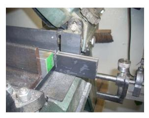
This V block sets the distance of the stop from the part being cut while permitting the stop to swing out of the way before cutting starts. Leaving the stop in place can cause jamming of the part against the saw blade which can cause unwanted shop excitement.
