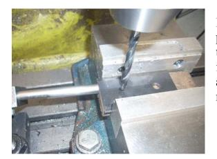
It is a simple matter to drop in the part, press it against the end stop and fixed jaw, tighten the vise, start the machine, drill the first hole, stop the machine, loosen the vise, and flip the part around. Then start the machine and drill the second hole.
