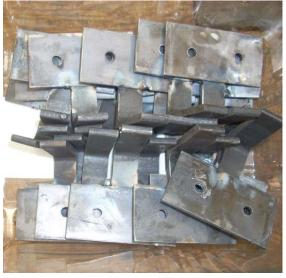
Even this simple fixture only makes sense if more than a few parts are to be made. Then it really speeds up the work and provides a high degree of consistency.
