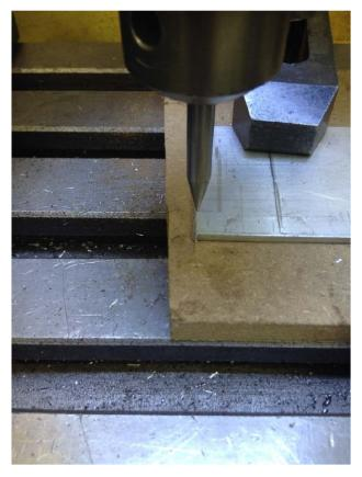
If accuracy is not that critical, I can use my spud. A few turns of the X axis crank and my edge is aligned with the point of the spud. This was my X = 0 location before moving the head and it is now true again.
