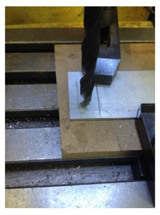
With the drill mounted, I have moved to a location .500" along the X and Y axis.
