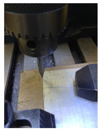
Next I need to set my Y = 0 point. If I had cut along the X axis, I could use the trick just presented with the end mill. But the edge I have is fine and is close enough to parallel with my X axis this time.
