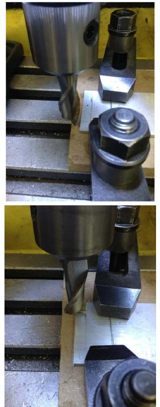
I will start back before my origin was first established. I have a piece of aluminum strap with straight side edges. I used the back edge to align the workpiece with the mill's X axis.
