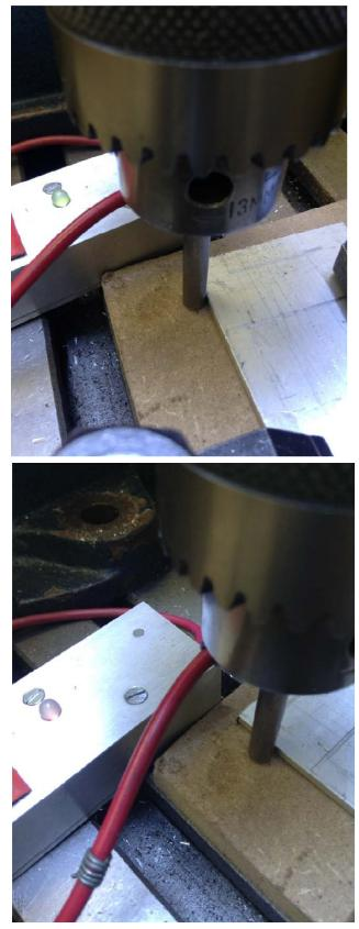
Another type of edge finder is an Electronic Edge Finder (EEF). The one I prefer is of my own design<sup>2</sup>. It was originally intended to be used on my lathe but has since shown to be useful on my mill too. I chuck up a piece of <sup>1</sup>/<sub>4</sub>" drill rod and
