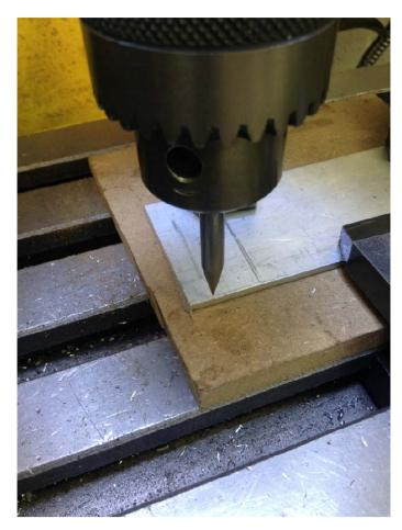
I repeated the procedure for the Y axis. The mill table was moved until the spud's point was directly over the edge.
