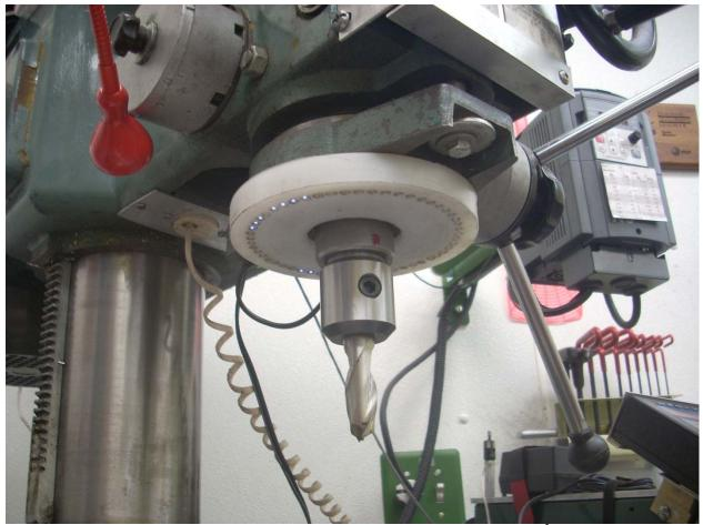
Here is the ring with the power just turned off. The power supply<sup>3</sup> that I used has a lot of energy storage inside of it so the LEDs stay on for about 30 seconds after I unplug it. You can see a few of the 54 LEDs still faintly lit.
