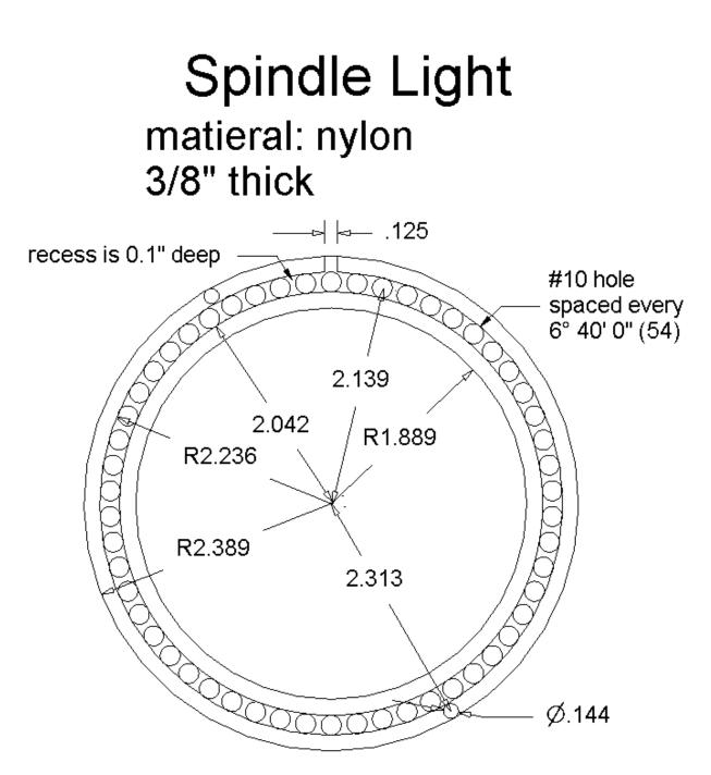
Ring holds 54 LEDs. The LEDs are grouped in sets of 9 in series with one 470 ohm resistor. All 6 strings are in parallel and powered by a 35V wall wart. Total current drain is about 100 mA
