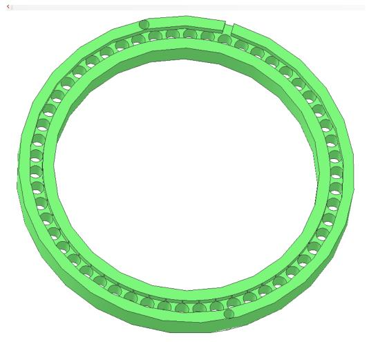
The ring was machined from nylon. There are 54 holes drilled with a #10 drill spaced equally around the bore. I originally planned to use a ring 3/8" thick but the piece I found in my scrap pile was 0.6" thick. This let me cut my channel a lot deeper and made it easy to put all resistors and connections inside. I then used heat glue to pot it all after testing.
