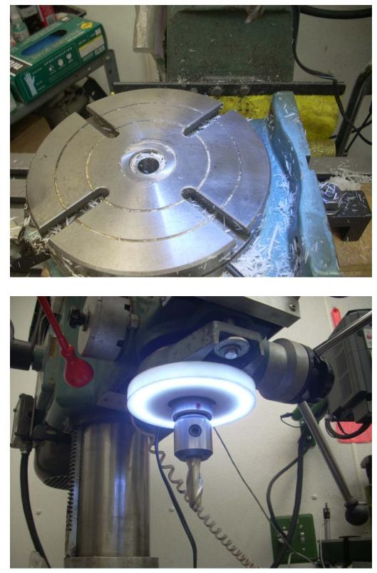
The light is uniform around the spindle and plenty bright.
