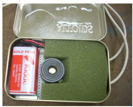
Open up the box and you find a 9V battery and a piezoelectric beeper. These beepers are so loud that no effort was made to cut a hole for the sound to get out. The green foam holds the circuit board in place.
