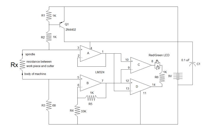
A variation on the design is to replace the piezoelectric beeper with a red/green LED. These LEDs could be positioned to shine on the feed dial making it easy to both monitor the dial's position and the circuit's state. In fact, the "body of machine" probe could be integrated with the LEDs so only two cables exit the device.
