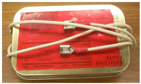
When not in use, the wires wrap around the box. Magnets at the ends of the wires stick to the box. The red tape prevents them from shorting together and turning on the device.
