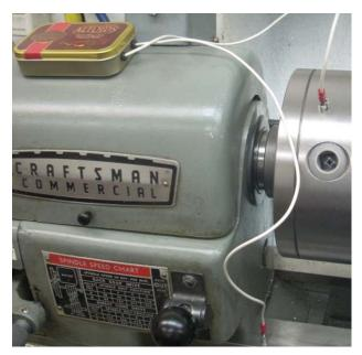
The second feature is the ease of use. Although there is electronics inside that Altoids<sup>®</sup> box, there is no power switch. Whenever I must deal with a power switch, it ends up being left in the "on" position and the battery goes dead. With this edge finder, power is on only when the wires are connected to the machine. And while power is on, there is a faint but rather annoying sound to remind me that the battery is being discharged.
