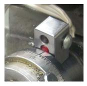
Once the cutter touches down, my Super Bright LED goes dark and my red LED comes on. Both LEDs go dark when they are removed from the lathe and placed back on the box.
