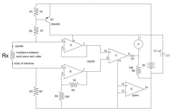
Op amp B measures the test current times R3. It then generates a small reference voltage which is applied to pin 9. The voltage applied to pin 10 is a function of both Rx and the test current. Op amp C compares two voltages that are both functions of the test current. In this way the test current's value drops out of the equation and the circuit is only comparing resistances.
