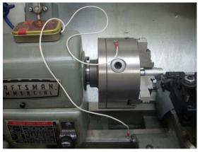
I connected the detector between my 3 jaw chuck and the ways and slowly fed in the cutter until I heard the loud beep. The longitudinal dial was then zeroed. I fed in again and made a small adjustment to the zero point.
