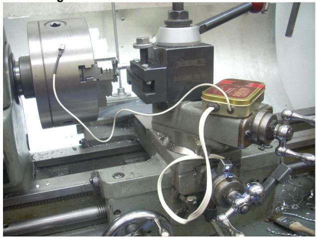
I have moved the two LEDs from inside the box into one of the magnetic clips. Now the LEDs can shine directly onto the dial.
