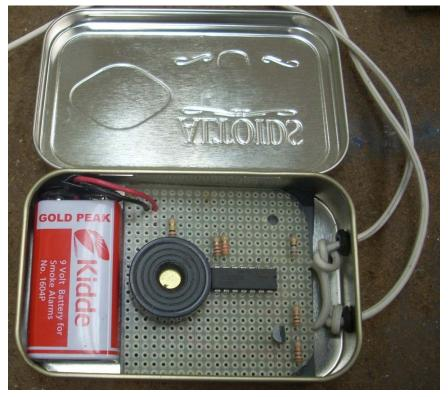
Under the foam is a circuit board with a small handful of parts in it<sup>3</sup>. Having all of this room made fabrication easier. All connections were made by directly soldering leads together.
