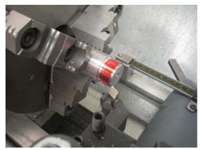
I backed out the cutter and coated the surface with dye.
