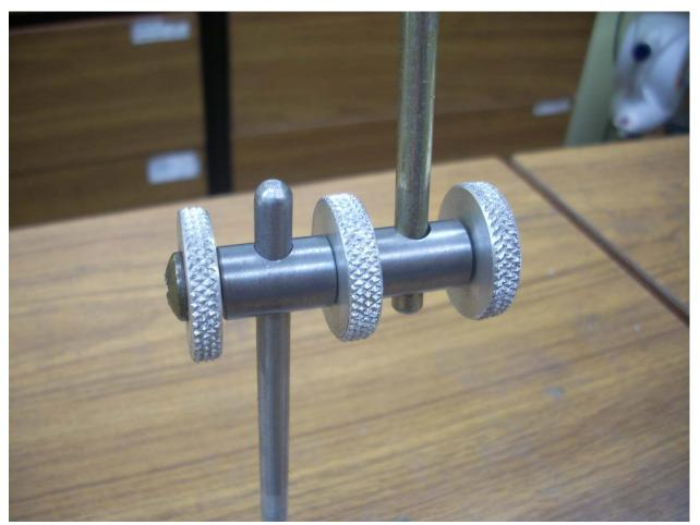
My initial tests indicate that this rod clamp will be useful. I plan to make a second one before I tear down my mill set up. If I was making a lot more of these clamps, I would set up a work piece stop in my lathe too.
