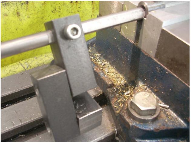
Since I was making more than one of these parts, it was worth my time to set up a stop on my mill. I then used my Digital Read-Out to locate the center of the part. I then drilled my cone shaped hole with my 1/4" spot drill and followed with a 1/4" drill. Then the second part was done with no further setup.
