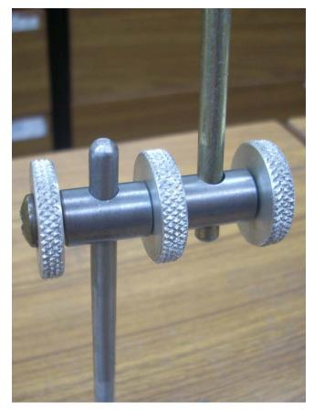
The outer knobs lock the ½" rod next to it. To change the angle formed between the rods, I loosen the knob in the middle.
