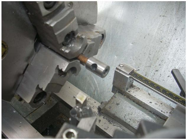
I polished the part by threading it onto a piece of ½-20 rod which acted as a mandrel.
