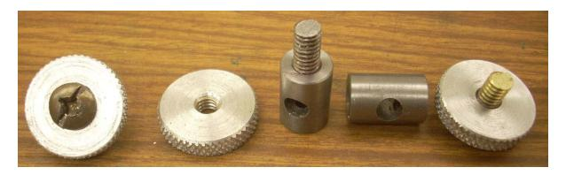
I screwed in my two brass bolts into the end knobs using Loctite Red. One of the bodies received the threaded steel rod and it too was glued in place. To get the spacing correct, I put a ¼" rod through the cross drilled hole, fed in until I hit it, and then backed out a little. Then came the hard part; leaving it alone for 2 hours while the glue set up.
