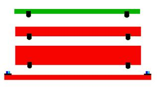
My approach is to secure the part being machined to a ½" thick slab of aluminum tooling plate. This plate would have an array of threaded holes that would be used with hold down clamps. The plate would also have close fitting ½" diameter pins that would provide alignment to the
