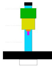
A round column mill/drill has one feature/limitation that drives many people crazy. When you raise or lower the head, it can rotate about the column. You then lose position on the table. The urge to fix this problem has hit just about every owner of this machine at some time. Sure you can avoid the loss of alignment most of the time with good planning plus avoiding extra long tooling. But it remains the "holy grail" of mill/drill fixes.
