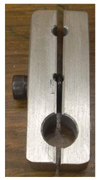
With the clamp assembled, you can see the gap between bars. The O-ring holds the bars apart plus prevents them from rotating when loose. If the bars flopped around while I was trying to fit the bars to it, the aggravation level would be far higher.
