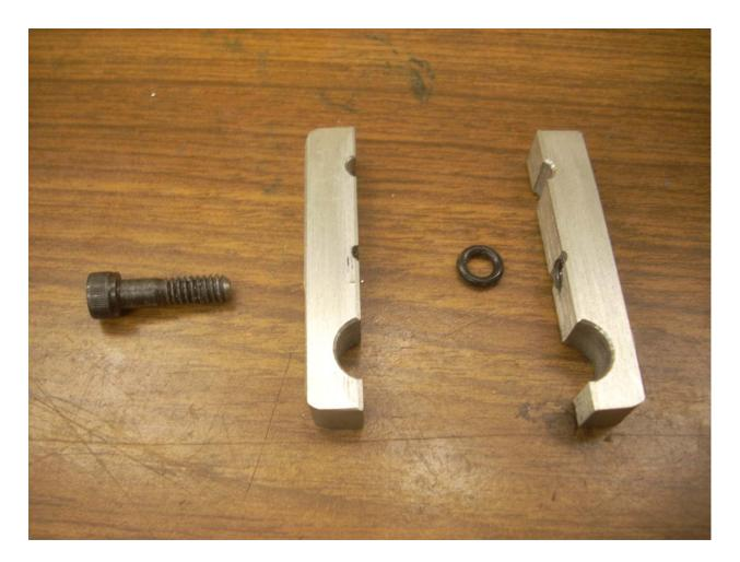
The clamp is made from four pieces. Starting on the right is my lower bar. An Oring fits over the screw on the left and makes handling this clamp much easier. The upper bar is almost a mirror image of the lower bar.
