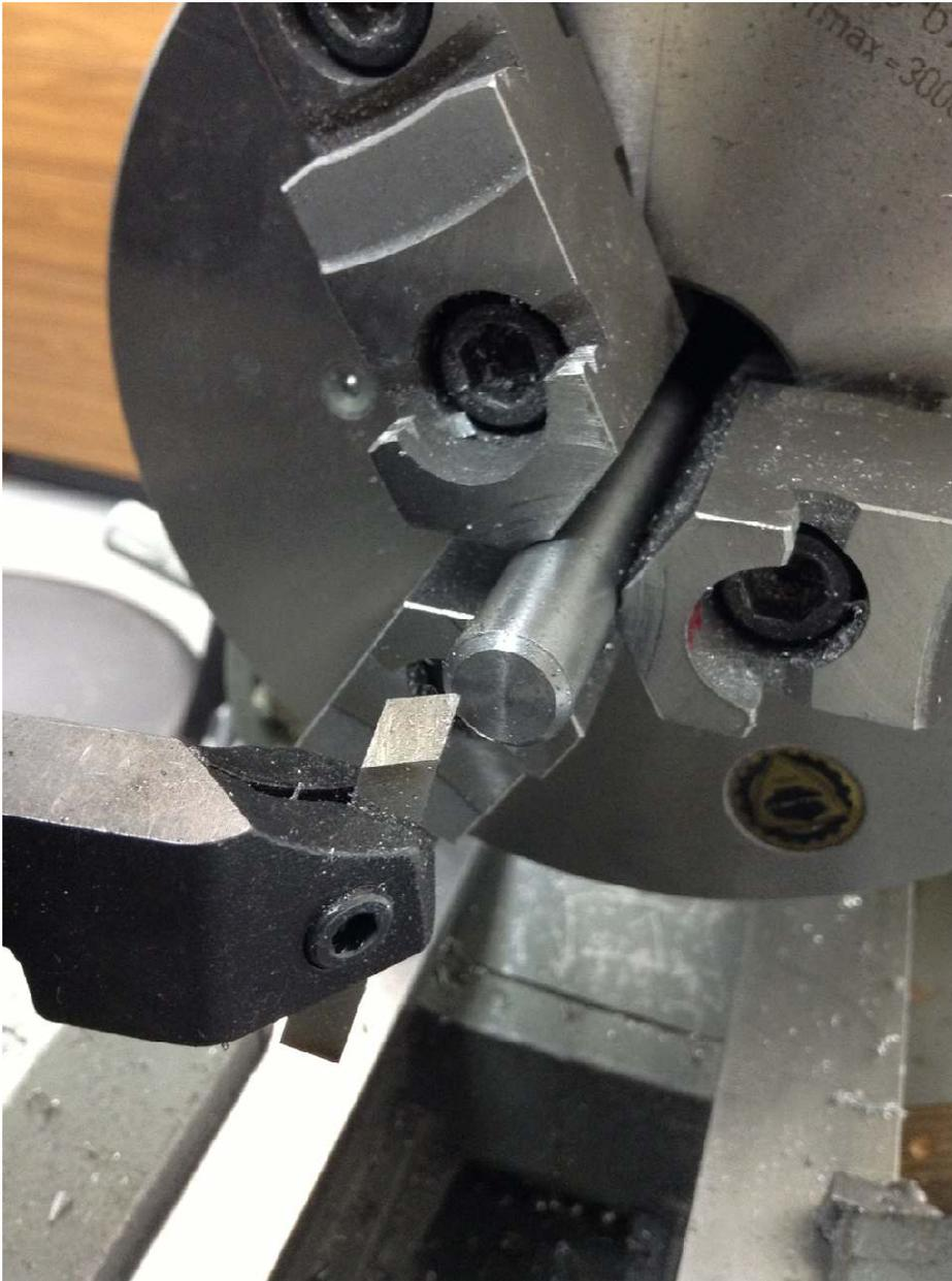
With the workpiece mounted in my 3 jaw chuck, I squared up the end and cut the bevel. The bevel looks nice plus prevents the top from mushrooming out from hammer blows.
