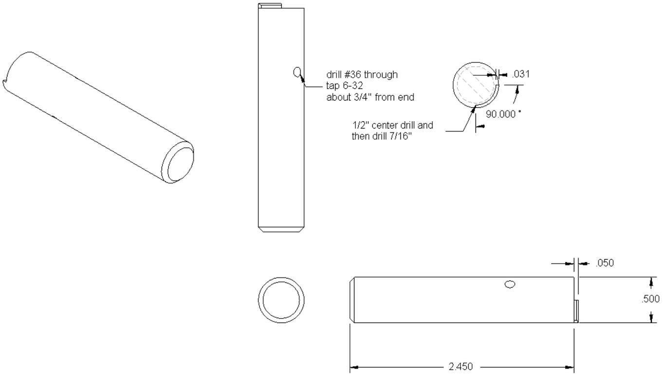
I made the punch from W-1 drill rod. This material already has a nice finish and machines well. I could have hardened the end of the punch but so far it seems to be holding an edge.
