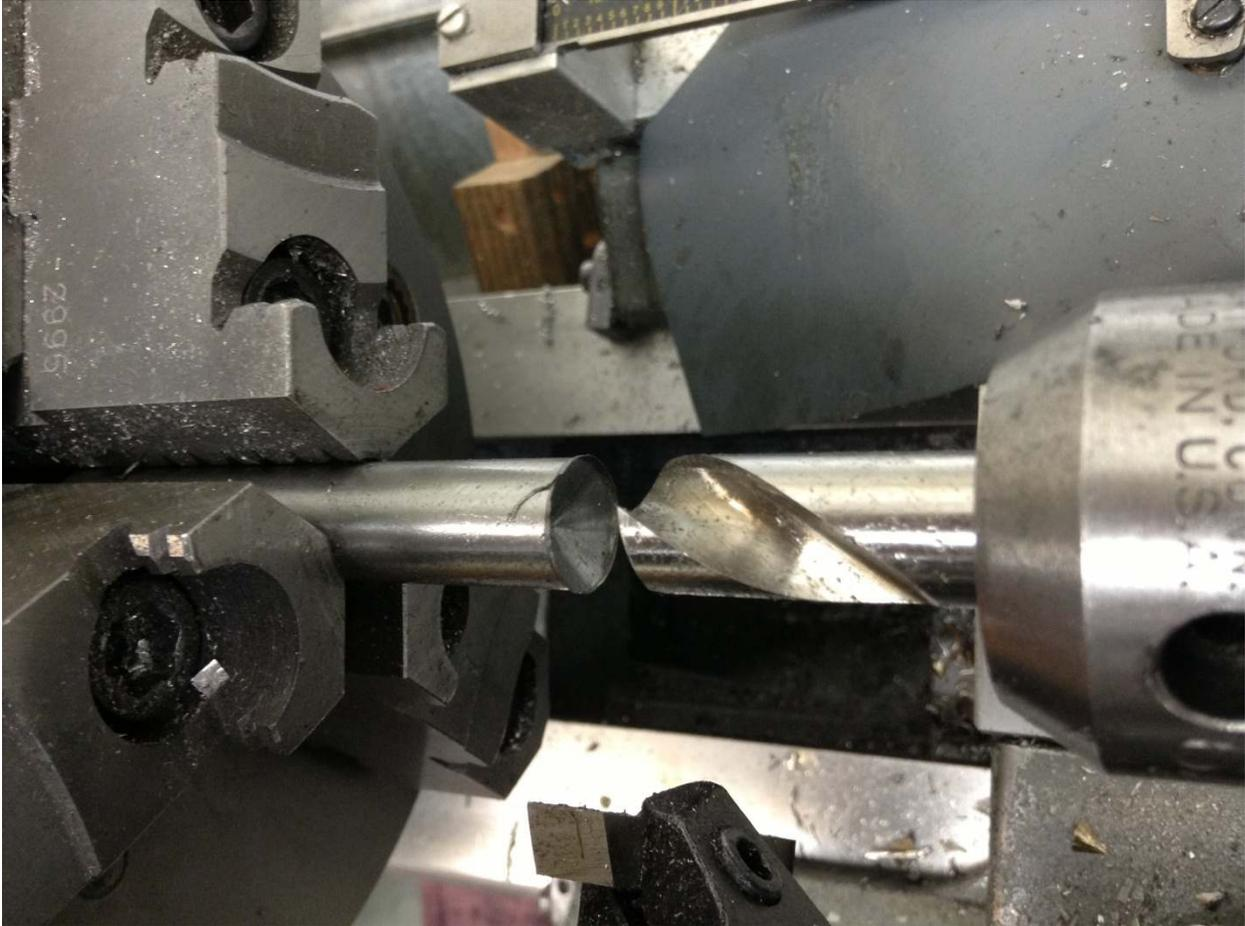
Next I used a 1/2" spotting drill to shape my cutting edge. Just feed in until there is no flat on the end of the stock. Not shown in the picture is the liberal use of cutting oil.
