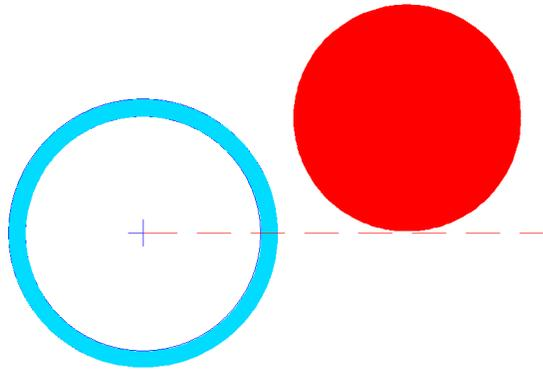
The end mill was moved along the X axis to the right of the workpiece. Then it was moved along the Y axis a distance equal to the radius of the workpiece minus about 0.01". And finally, the end mill was lowered down by about 0.04".
