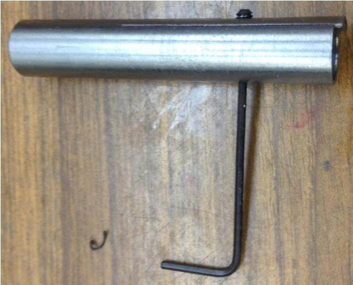
After drilling and tapping, I adjusted the set screw so it extended out the side of the workpiece with the cutter. Then the punch was placed in the V block and the set screw adjusted to prevent any rotation.
