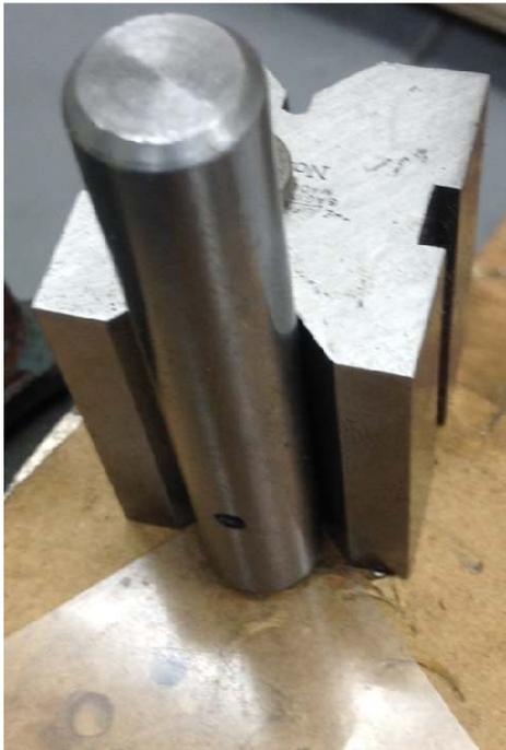
Then the punch was placed in the V. A quick tap with a ball peen hammer is all it takes.
