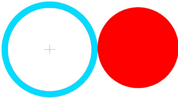
On the far left is an end view of the partially finished cutter. The blue is the cutting edge. On the right is the end mill. I started, with the machine off, by touching the end mill to the side of the workpiece. I then set my X axis to zero.
