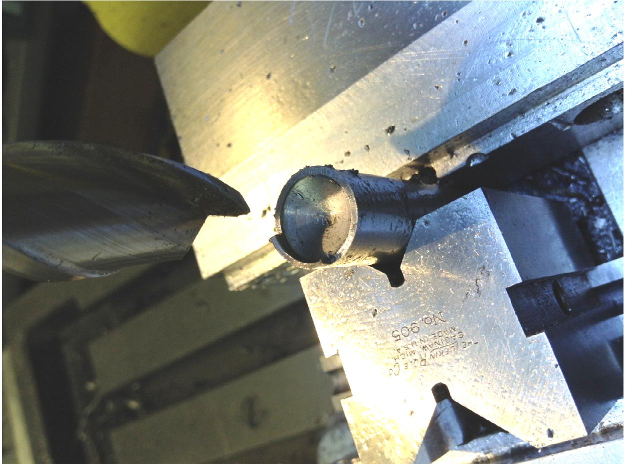
Next stop was the mill. I cut off all of the end except for a 90° segment. The depth is about 0.05".
