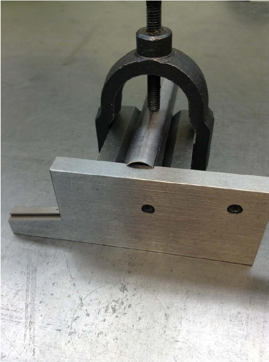
I used an adjustable parallel under the lip of the punch to align it on my V block. I was then ready to drill my set screw hole and have it centered on this cutting edge.
