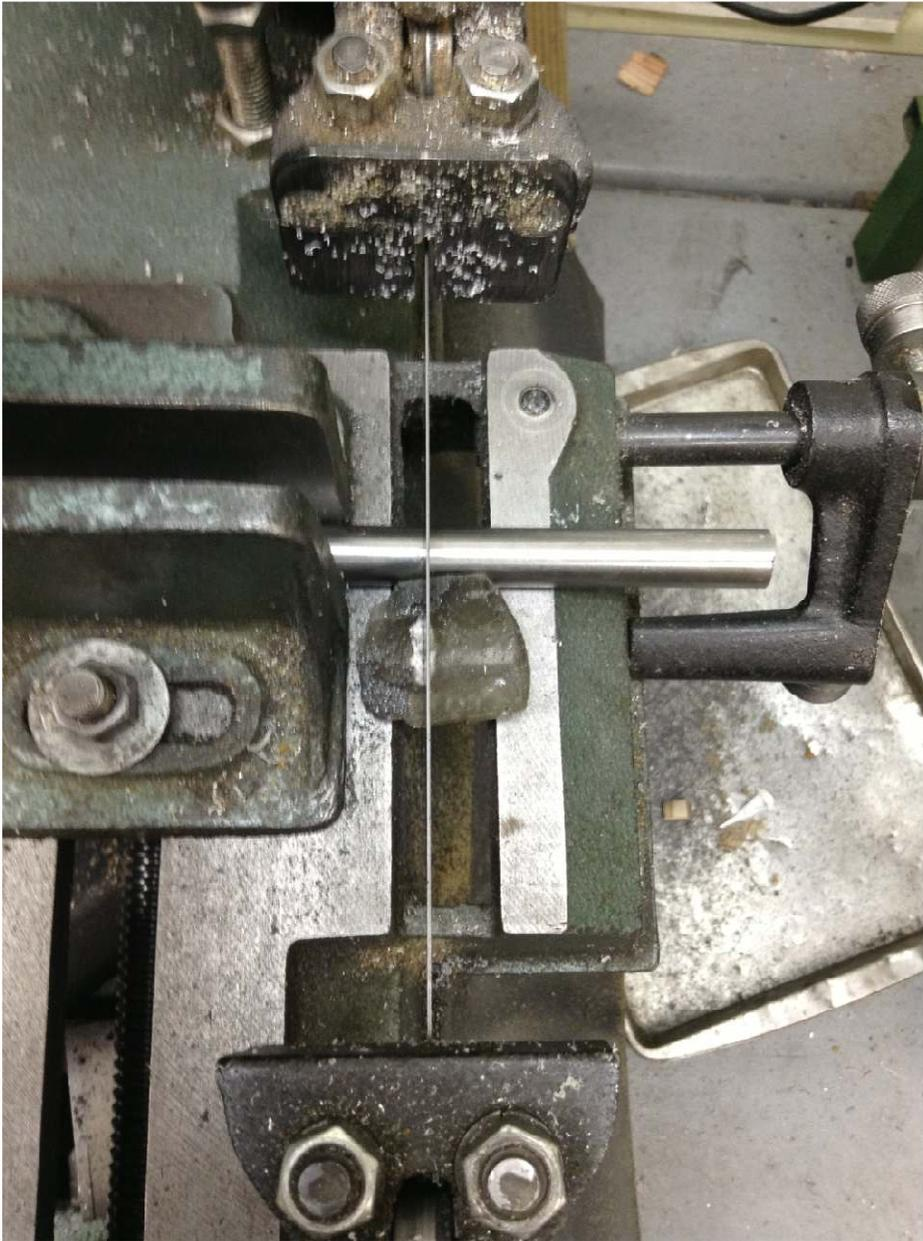
The first step was to cut off a 2 ½" long piece of the drill rod. I used a chunk of paraffin wax as my cutting "fluid".
