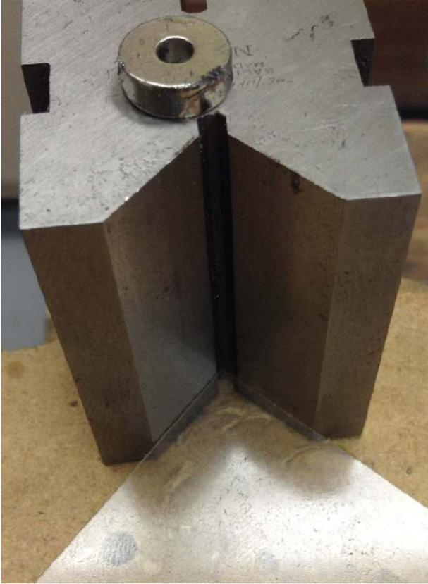
I placed the plastic to be cut on a piece of scrap Medium Density Fiberboard (MDF). The corner of the plastic was aligned in the V.
