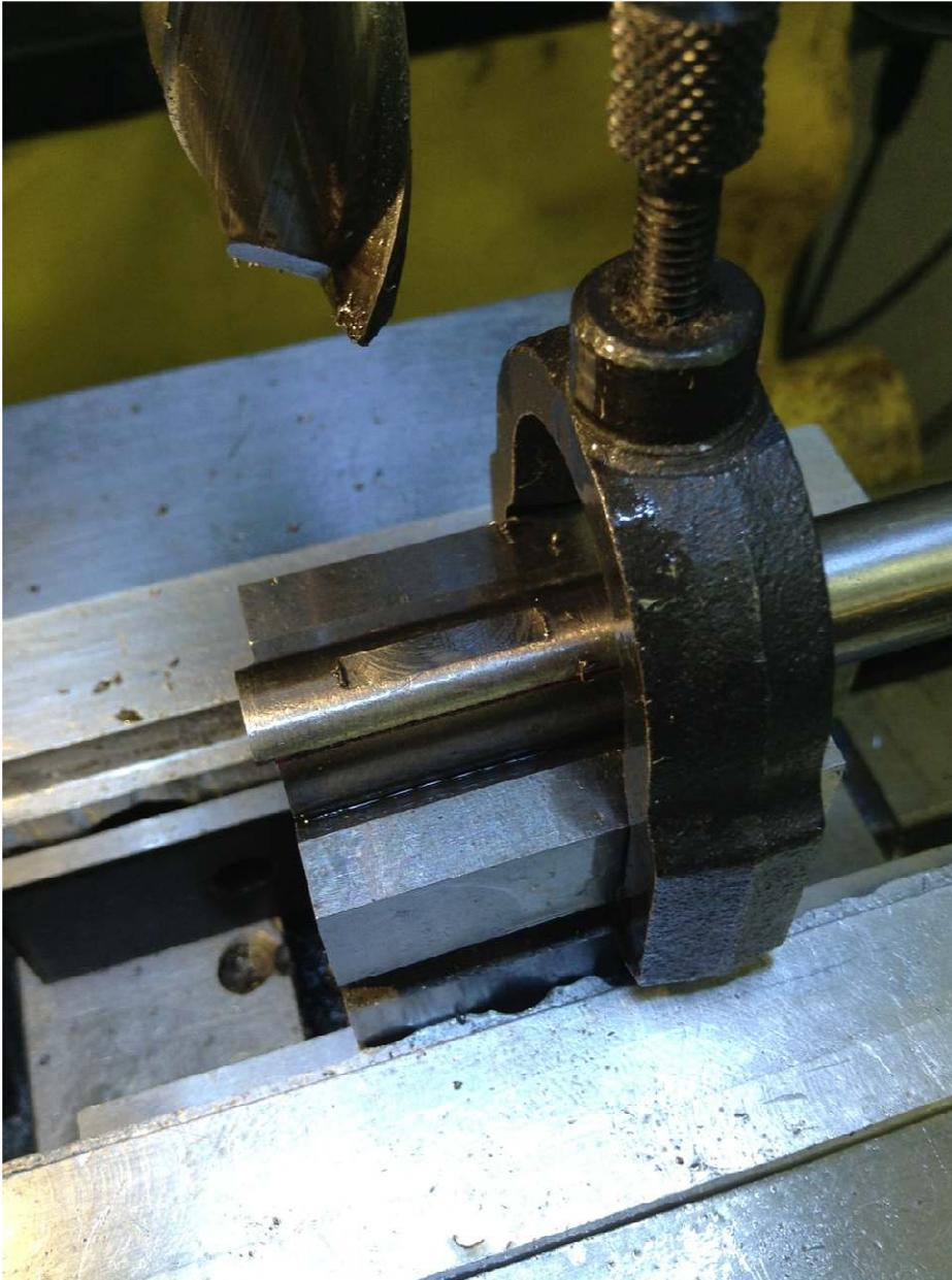
I still had my end mill mounted so first cut a flat in the flank of the workpiece. This made it easier to verify I was on center.
