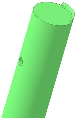
The cutting edge is a 90° sliver. The set screw hole has been aligned to bisect the cutter. This puts the corner of the plastic to be cut in the center of the cutting edge.
