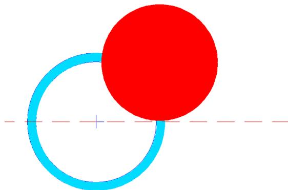
With the mill running at this RPM, I feed the cutter along the X axis. Note that I am 0.01" away from the final cut surfaces. This let me perform my "roughing cut". After feeding all the way across, I moved the cutter along the Y axis so I am right at the dashed red line plus feed down on the Z axis so I am 0.05" below my zero point. I then removed only 0.01" of material and took my "finish" cut.
