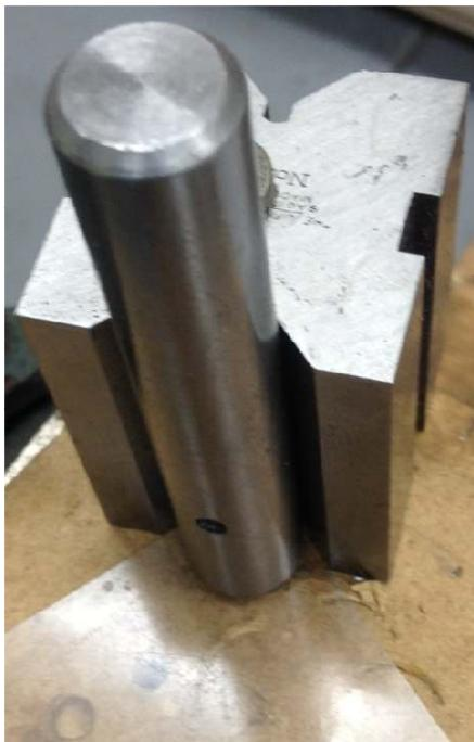
Here is the finished punch placed up against a V block. The V block performs two functions. First, it aligns the corner of the plastic directly below the punch. And second, it holds the punch in the right position.
