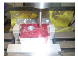
With the spud again in the drill chuck, I moved on to the chain drilling line.
