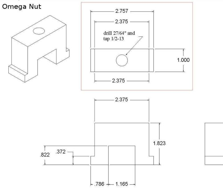
The dimensions shown in this drawing are for my RF30 mill/drill. I simply measured my T-slot and spacing and then subtracted 0.04" from each dimension. This gave me 0.02" of clearance between all mill table surfaces and the Omega nut. The overall height of the Omega nut, at 1.823" is arbitrary. If you are using 2" bar stock, make the height 2". All critical measurements are from the bottom surface.
