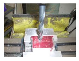
I then followed with my 1/2" drill. It was harder to drill the 1/4" hole than the 1/2" hole. The 1/2" drill sailed right through.
