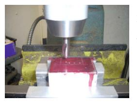
I used my spotting drill to cut a shallow cone into the surface. This prevents the drill from wandering around the surface before it starts to cut.
