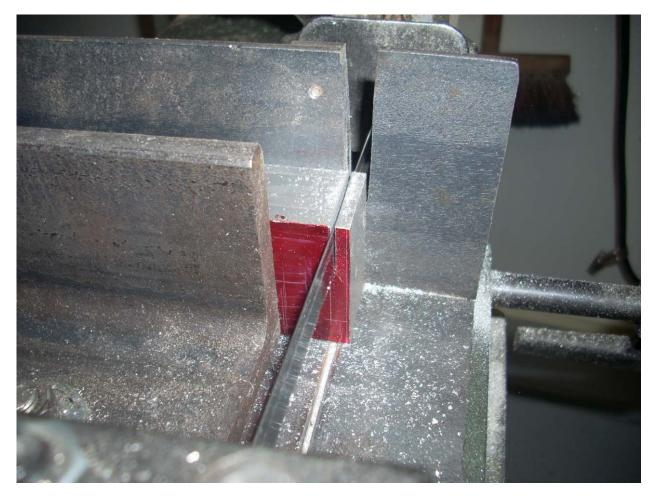
With the block on end, I made my second cut to rough form the first ear of the Omega nut.
