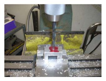
After using my spotting drill, I drilled a 1/4" hole. This was followed with my 27/64" drill which is specified as the correct tap hole for a 1/2-13 thread.
