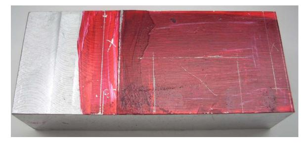
On the far left side is where my saw will cut off the unused part of the block. Note that I have scratched "X" in areas to be removed. My hope is to prevent really dumb mistakes.
