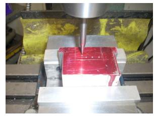
Then I use my spud to set the center of rotation at the center of the 1/2" hole. In order to make it easier to see, I have used a layout punch to mark the hole centers.
