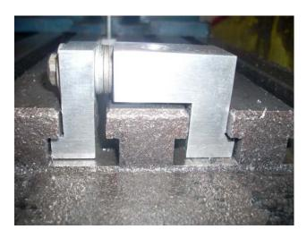
That left leg would be a real problem give how little it engages the T-slot. Since this is a prototype, I sawed that left leg off and added a spacer. A bolt was used to reattached it. Not pretty but it lets me try the Omega nut out with less risk to the T-slot.
