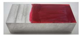
My first step was to find a bar of aluminum a little larger than the finished Omega nut. I then painted the top surface with red dye in preparation for layout lines. The bottom face was smooth so I used it for my reference surface. The right end was a little ragged so I
