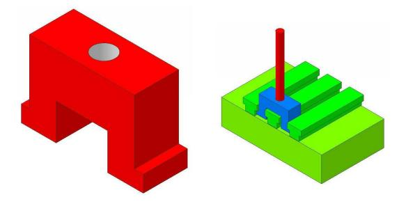
An "Omega nut" is a variation on the idea of a T-nut. While a T-nut slides into a Tslot on a mill table, an Omega-nut slides into two adjacent T-slots and straddles the island between them. Most of the time, a T-nut works just fine as an anchor point for a threaded rod. But once in a while I want my anchor point to be half a T-slot over. That is when the Omega nut is handy.
