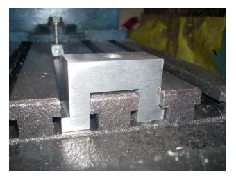
I have placed the prototype Omega nut into the T-slots. My error is now very clear. The left leg is too thin which causes an excessive gap between it and the left T slot overhang. After much head scratching, I traced the problem back to a mistake in my drawing. Lesson re-learned: verify the drawing against reality. Can't win for losing...
