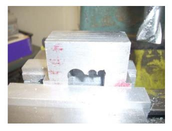
The ears have been milled along with the top surface. Here is one of those bone headed moves that I make far too often. I mounted the block with the layout lines facing away from me! I am using a Digital Read-Out (DRO) to position my end mill but the layout lines keep me from making those big mistakes.
