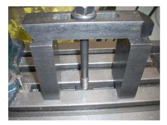
Contrast that with the use of a T-nut. Here the support blocks span the Tslot. Now, these support blocks are wide so this is not an issue. But I have had cases where the blocks had to be turned 90° causing the blocks to be just partially supported by the overhang of the T-slot. If a slightly thinner support block was needed, it might jam into the T-slot.
