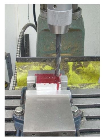
Sawing out the inside is not as straightforward. I can saw straight down on both sides but the last cut has no room for the saw to enter. Instead, I drilled a 1/2" hole near one inside corner and chain drilled with 1/4" drills the rest of the way. I'll say more on this later.
