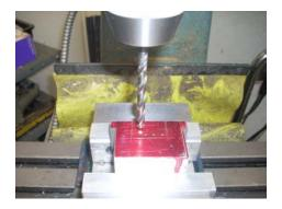
I started by drilling a 1/4" hole. Rather than one hard push through the block, I "pecked" at it. I drilled down about 1/4" and then retracted the drill to bring up chips. This process was repeated until I was all the way through the 1" block.
