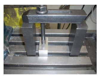
Here is the Omega nut in use. Note that the support blocks are resting on the island between T-slots.
