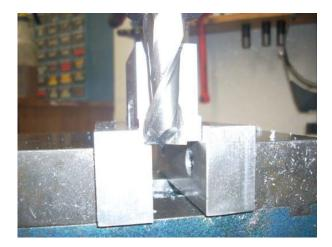
I have clamped the block into the soft jaws of my vise. With the end mill sitting on the horizontal surface of my soft jaw, I set my Z axis to zero. Consistent with my drawing, all height measurements will be relative to this bottom surface.
