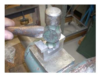
The final step is to spoil the last thread in the hole to prevent the threaded rod from feeding through and marring the mill table. I took a small ball peen hammer and fitted the rounded head into the hole. The part is solidly supported on the anvil of my vise. I then struck the face of the hammer with my lead hammer. The result was a nicely formed cone with that last thread crushed into the one below it. Do not try this with a hardened faced hammer as it can shatter one or both
