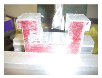
I then removed the part, deburred it, cleaned the clamping surfaces on my soft jaws, and mounted the part upside down. My reference surface is now facing up.
