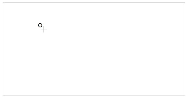
Here I have a dead flat surface (a plane), with a single point on it. I have marked this point with a cross hair and named it "O" for Origin. All measurements will be relative to this point.
