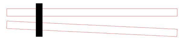
Say I bore a second hole in the block and fit a second rod. If this new hole is "much" larger than the rod, then the rods do not have to be parallel yet the block can move along the rods. The tighter the fit between new hole and its rod, the closer to parallel must be the rods.
