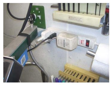
To the right of my mill I have added a power strip with switch. The wall wart to the left is for the spot light.
