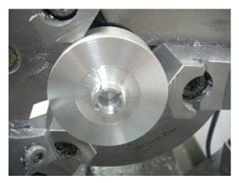
I'm back on the lathe now. A piece of aluminum round stock slightly smaller in diameter than the washer blank has been chucked up. I turned down a length about 0.1" longer than the rough thickness of the washer to a diameter of 0.500 + 0, - 0.004". I also cut a recess around this smaller diameter so the washer will not come into contact with the small radius at the bottom. The rest of the face has been lightly cut
