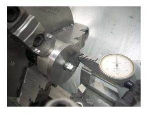
I used two instruments in order to see what was going on. The first was a Dial Test Indictor (DTI) that could sense variations in the outside face of the washer. The second was my micrometer.
