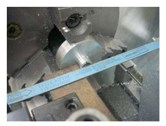
After tapping the hole, I can finally show you how I cut the slots. I clamped a piece of scrap MDF into a spare Quick Change Tool Post tool holder. The height was set such that when I put a hacksaw blade on the MDF, it was on the centerline. It was then a simple matter to saw down to my reference surface. The part was turned about 90° and a second cut made.
