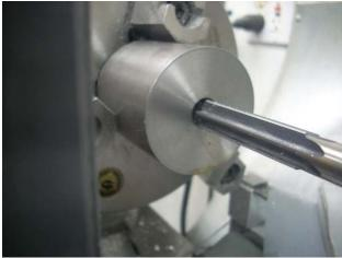
I next ran a 1/2" reamer through the hole. The washer might not need this precise a hole but my fixture will.
