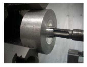
I next drill a 21/64" pilot hole for a 1/8 -27 N.T.P. pipe tap. The tap is tapered which means that when I screw in this stud, the diameter of the turned 1/2" part will expand. This expansion will lock the washer in place.
