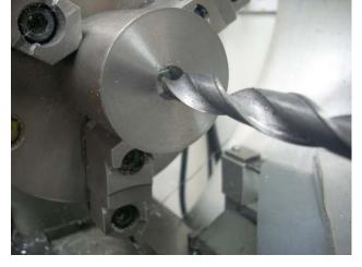
I used a 1/4", 3/8", and 31/64" drill to a depth of about 1/2" for a 0.2" thick washer. I want to be sure that the cone in the bottom of the hole is not within the washer blank being made.
