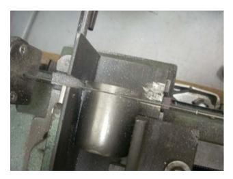
I removed the bar from the chuck and clamped it into my band saw. The roughed out washer is sliced off. I then used a deburring tool to clean up the 1/2" hole
