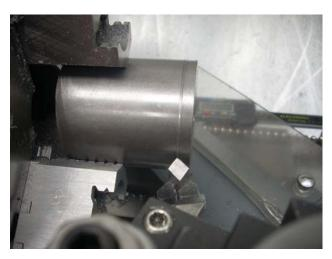
I then cut a groove about 0.05" beyond the finished thickness of the washer. It will help me to set my band saw blade in the right location.
