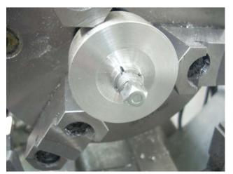
Here is the finished mandrel with plug installed. Its accuracy is only present until it is removed from the chuck. If you do remove the mandrel, you will have to reface it and possibly re-cut the 1/2" part. Worst case, you will have to make a new one.
