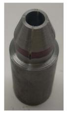
I am left with a neat slab of caulk between each jaw of the collet. The rough saw cuts give the caulk plenty to grab.
