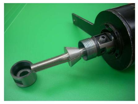
Here I've got a tap being held by its flex collet. The tapping head on the right has a matching taper. As the nut, shown on the left, is tightened, the flex collet is compressed and tightly grabs the tap's shank.
