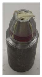
This is the fun part. I squirted 100% silicone caulk into the blind hole and followed by slowly pressing in the shank end of the drill used to make the hole. I then removed the excess from the outside of the part. Inspect each cut to be sure it is completely filled.
