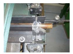
I cut a 3" piece of mild steel that was slightly larger in diameter than the collet. This will let me make all three collets plus have plenty to grab in my lathe chuck.
