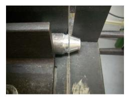
I then sawed the part off the bar. Using a belt sander I smoothed the end plus did my best to square it up. The shallow parting cut helped me see where to remove metal. Note I am left with the end of the bar stock ready to make the next collet. The outside diameter has been cut so I only need to cut more of it to get back to about 1" of length. The centering hole for the next larger size is also in place along with the start of my two saw cuts.
