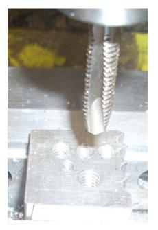
As a test, I have drilled a tap hole and run my 5/16 - 18 tap through it. It performed just as well as my 1/4 - 20 tap held in a real Jacobs Flex collet.
