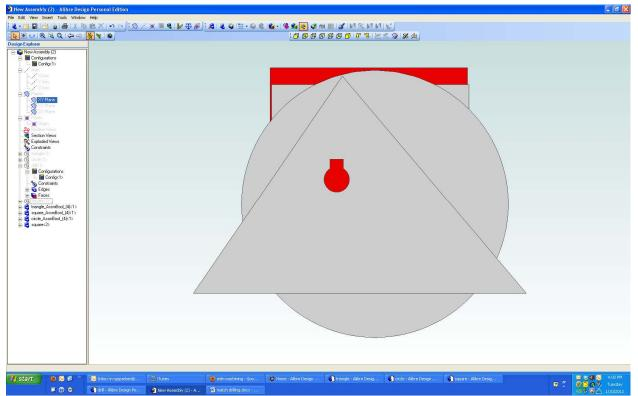
To illustrate how an object that has been "drilled" is now separate from its parent object, I have brought in a second copy of my square, changed its color to red, and put it behind the three gray objects.
