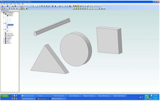
I first created three shapes that are each 0.5" thick. The forth object is my "drill". It does not have to be round for Alibre to form the matching hole. So I guess you can think of it more like Electrical Discharge Machining than drilling.
