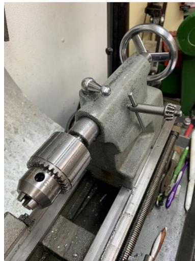
During set up, I can stick the chuck key to the side of my tailstock. When done, it goes back on the shelf.
