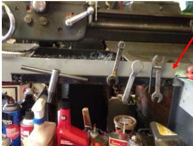
A second magnetized bar on the front of his lathe holds numerous tools that must be quickly accessed and then stored. No need to aim for a holder, just put the tool near this bar and it is held fast.
