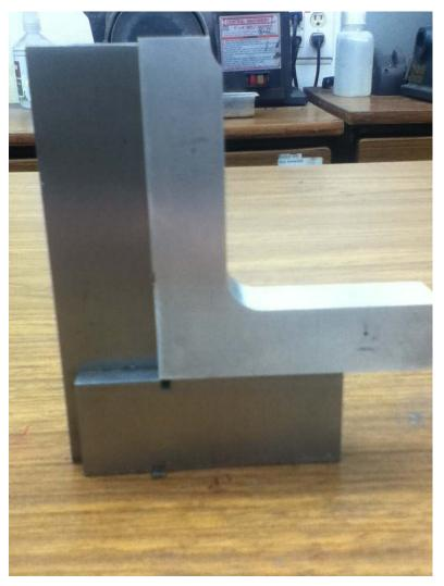
The last parameter to assess is the angle between the legs of the bracket. A quick and simple test is to place a known accurate square next to the part and look for light pass thing through gaps in the edges. I saw no light so this is a decent fit. A better assessment would involve a surface plate and a Dial Test Indicator. Let's leave that for another day.
