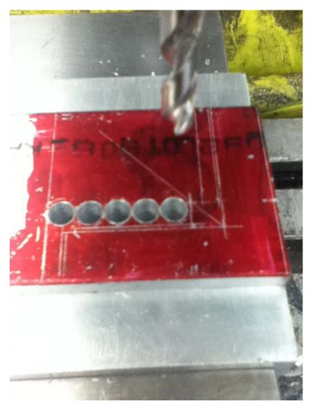
The <sup>1</sup>/<sub>4</sub>" drill was freshly sharpened on my Drill Doctor<sup>®</sup> so easily cuts through the plate. Note that the edges of the holes touch the rough cut line. I have scribed the hole center for the other leg but will use my bandsaw on the rough cut line instead.
