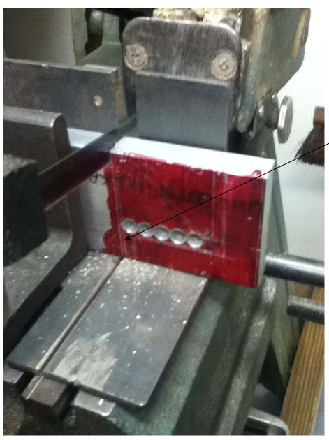
The total work is reduced by using my bandsaw because I don't need to chain drill first.
