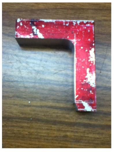
I removed the part from the mill in preparation for final deburring. Except for the one screw up, the part seems to be fine. But does it really meet the Fit and Finish requirement? In my case – yes since my goal is just to demonstrate technique. But how close to the plan did I get? The last phase of the work will answer that question. It is time to do an evaluation of the part.
