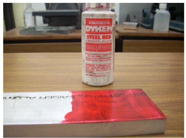
I could take a sharp knife and scribe lines directly on the raw metal. The problem is that the contrast is poor unless these lines are cut deep. Instead, I use a layout fluid which is painted on the surface and left to dry for a few minutes.
