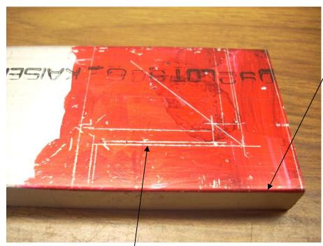
The bottom of the horizontal foot will ideally be the original edge of the plate. But if the plate is not perfectly aligned to my mill's axes, some cutting will be necessary to square up the part.
