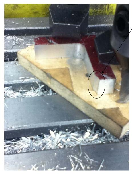
This is after the finish cut. You can clearly see that I almost got it right. The instant I fed in the cutter at what really was the right point (2"), I saw that I had taken a very big cut. I quickly backed out and then saw the wrong finish line so cut to it. This would have been fine if I had just realized which was the true finish line.
