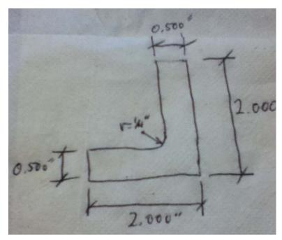
It is time to move from theory to practice. My goal is to make an aluminum 2" by 2" bracket with a 1/2" square cross section and a 1/4" radius in the inside corner. This rough figure satisfies my need for a clear picture. Although I do show 3 place accuracy to the right of the decimal, I really have not decided what I want yet.
