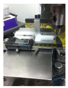
I could see that I had 0.247" to go. Two passes of 0.100" each got me down to about 0.05". Then I made a 0.030" pass before checking with the caliper again. The caliper showed I had 0.014" to go. I then took my first, calibrating, finish cut of 0.007". The caliper said I now had 0.007" to go. This told me that there was no need for a correction factor. I then dialed in my final 0.007" cut.
