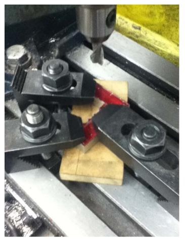
We are finally ready to run the mill. Since the inside corner is to have a 1/4" radius, I will use my 1/2" diameter end mill. It is mounted in an end mill holder which makes it convenient to install into my spindle.
