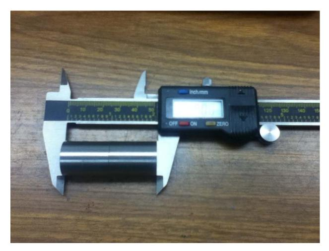
I also own a cheap Harbor Freight digital caliper. I zeroed the caliper on the two spacer blocks. In this way the readout will show me differences from 2.000". The caliper has its own error but experience has shown me that this error is small when movement is small. I am only expecting an answer to the nearest 0.001".
