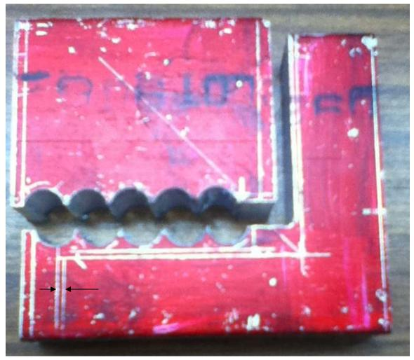
With the roughed out part free from the plate, I am ready to start milling. The left end rough and finish cut lines are clearly visible. I just didn't see them!
