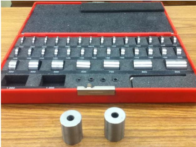
I own a set of what are called Spacer Blocks. These cylinders have a length accurate to +/-0.0002". I have removed two 1.000" blocks.
