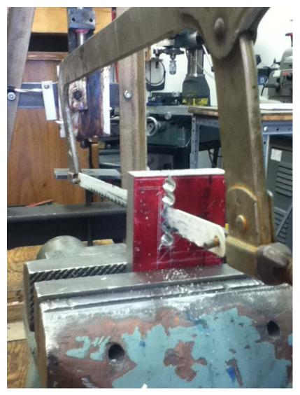
I'm using a 24 teeth per inch hacksaw blade to cut the web. It only takes one or two passes to clear each web.
