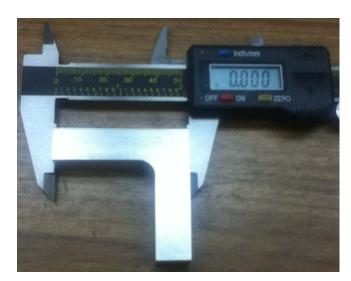
After deburring, I did a final check with the caliper. Now, that's a lot closer than being 0.251" off!
