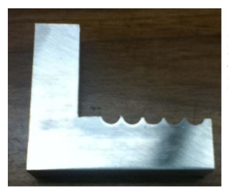
All of that drilling and sawing has raised burrs on the back side of the roughed out part. I used my belt sander to smooth the surface.
