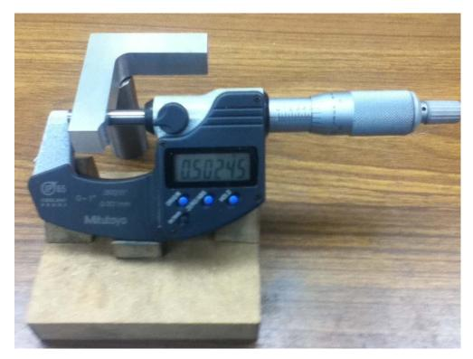
My first test is for the thickness of the longer leg. My micrometer is good to  $\pm$ -0.00005" and has been zeroed before use. I read 0.50245" so am 0.00245" too thick at this point. The test was repeated at two other spots along this leg and a maximum variation of 0.00015" was seen. I then repeated the test on the short leg and saw 0.050340" at the end with a maximum variation of 0.00015". The absolute thickness error of 0.002" or 0.003" could easily be improved. The variation is good
