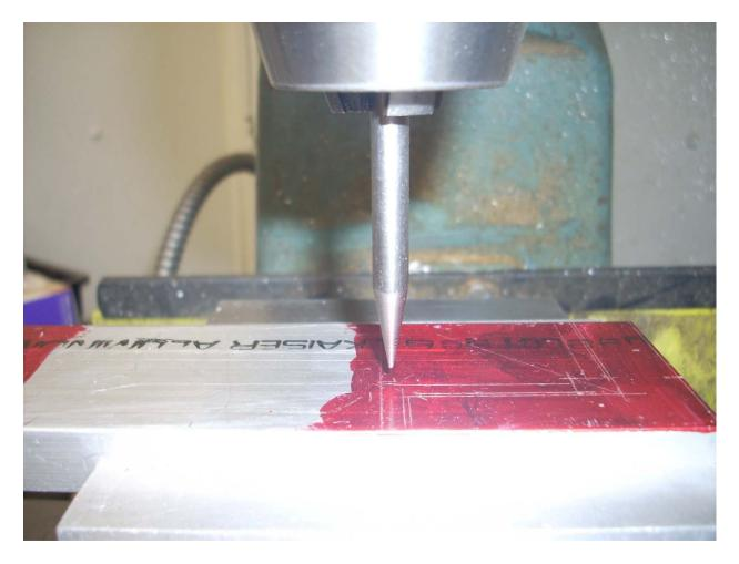
I have placed the plate into my vise and am using a "spud" to locate the drill chuck's center of rotation on the chain drill scribed line.
