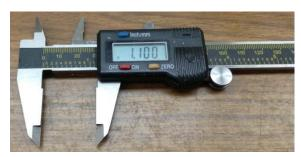
It is standard practice, if you own a digital caliper, to zero the display at the diameter you want to reach. Here I have zeroed the caliper with the jaws closed and then moved them apart until I read 1.100".
