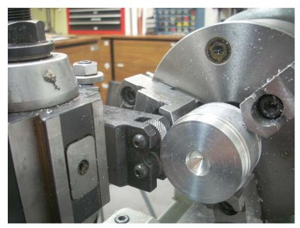
I was using a knurling tool that came with my Phase II Quick Change Tool Post.
