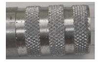
Here you see three test passes in aluminum. The one on the right and middle match the guidelines in Machiniery's Handbook. The one on the left is as far from the correct value as it physically possible. Yet they all came out looking the same.
