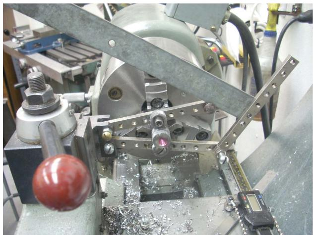
My proof of concept machine used the existing knurling wheels and the body of the QCTP knurling support. I added a few bits from my scrap bin and screws. My first attempt at knurling was on 5/8" diameter 12L14 and it worked perfectly. I then tried it on some 2 <sup>1</sup>/<sub>4</sub>" 12L14 and got the same great result.
