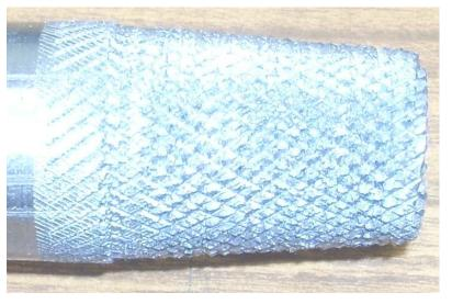
This sample was formed in 12L14 leaded steel. After many attempts to find the exact diameter that will give a screwed up knurl, I decided to cut a 2.5° taper and then run the knurling tool along that taper. If the dominant variable in knurling was the diameter of the work piece, then I expect the pattern to vary from poor to perfect and then back to poor.
