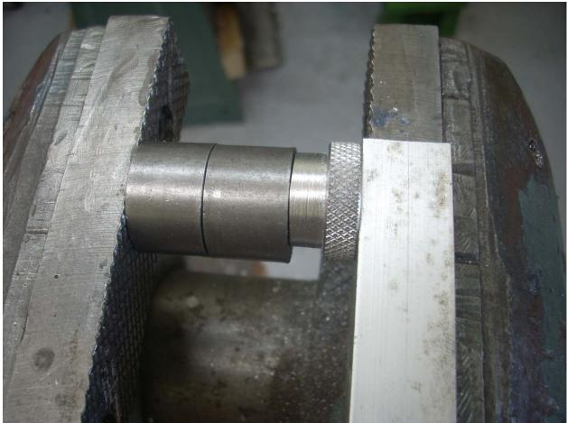
A few turns of the handle and the head has been pressed into the knob.
