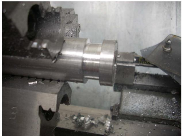
I fed the cut off tool in twice in order to cut the 0.800" diameter a bit longer than called for. This gives me room for my saw.
