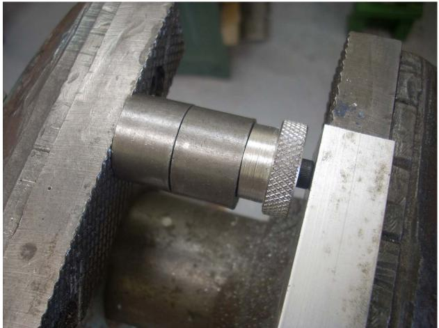
Nothing fancy here. I'm using my bench vise to apply the pressure. A piece of aluminum covers the jaw so the top of the screw head is not marred.
