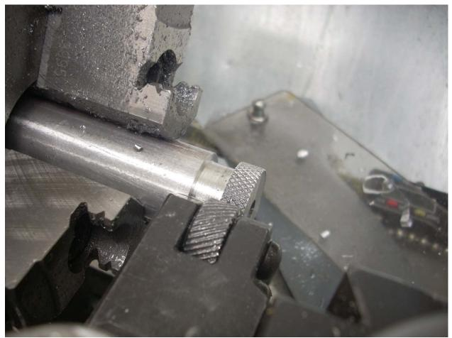
With my knurling tool mounted, I fed it into my part with lots of cutting fluid flowing. Feed in slowly and do not disengage until done. You can turn the lathe off, inspect, and turn it back on. If the knurling does not come out clear, you may have a knurling tool that is not compatible with a 1" diameter cylinder. You may need to turn the cylinder down to a smaller diameter to get proper forming.
