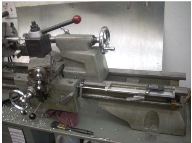
I then use my digital caliper that is clamped to the ways to precisely move the apron 0.70". Then when I feed the drill in, I stop when the jaw hits the stop and I have a hole that is 0.70" deep measuring just the straight sided part of the hole. This particular hole does not have to be precise; I'm just showing how it all works.
