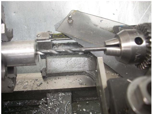
I drilled my small hole first to a depth of about 0.7". Do you see that cut-off tool that is near the jaws of the drill chuck? I'm using that as my depth stop.
