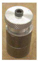
The screw is all the way through. I have placed the knob on a stack of steel cylinders in preparation for pressing in the head.
