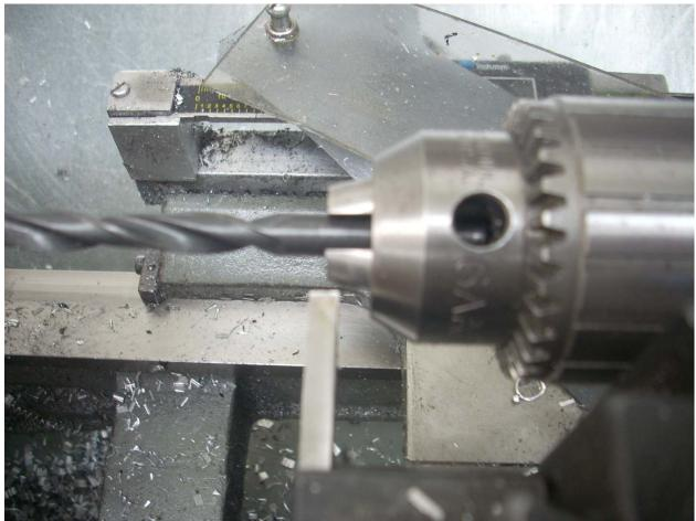
With the 3/16" hole drilled, my "N" drill has less metal to remove. I am again using my cut off tool to set the depth. This hole does have to be a bit more precise. I want to go in 0.200" from the surface.
