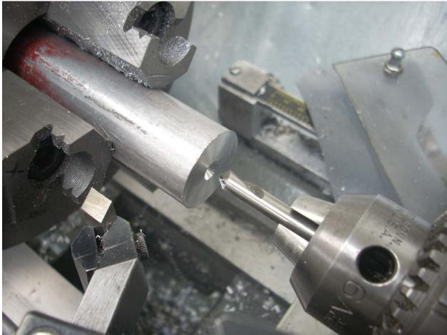
After facing the end with my cutter, I used a spotting tool to cut a cone shaped hole in the end. This helps the drill to stay centered.
