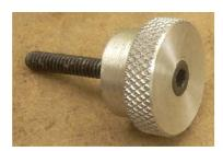
If you can't get the head to press in, use the next larger size drill for the large hole. If the head does not hold, make a new knob and go with a drill one size smaller. You might be able to salvage the knob by using Loctite<sup>®</sup> Red to glue it in place.
