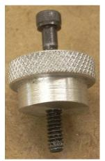
The 10-24 SHCS has been threaded down the hole. The hole is just a bit smaller than a clearance hole so the screw easily cuts its own thread.
