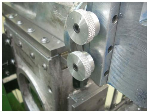
I have a number of Socket Head **Cap Screws** (SHCS) that must be adjusted periodically. Not much force is needed but I had to reach for an Allen wrench every time. In most of these applications, a 1" diameter knob would be fine. The way the knob has been
