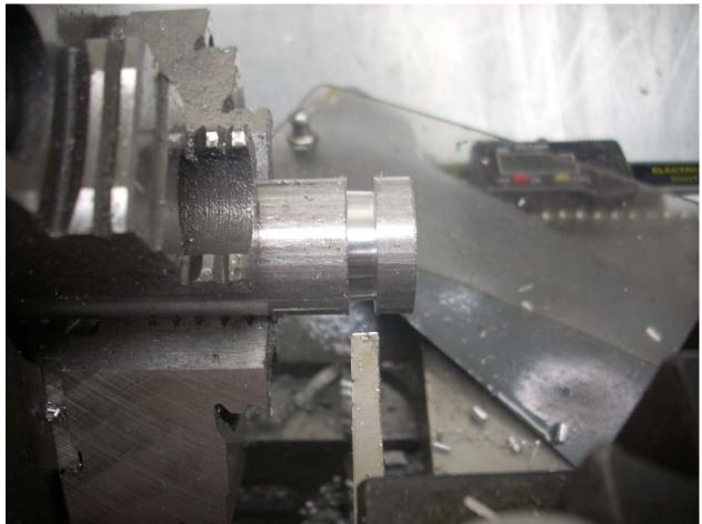
Here I'm actually using my cut off tool for cutting. I moved over 0.250" and fed in 0.100" from the surface. This will give me the 0.800" diameter called out in the shop drawing.
