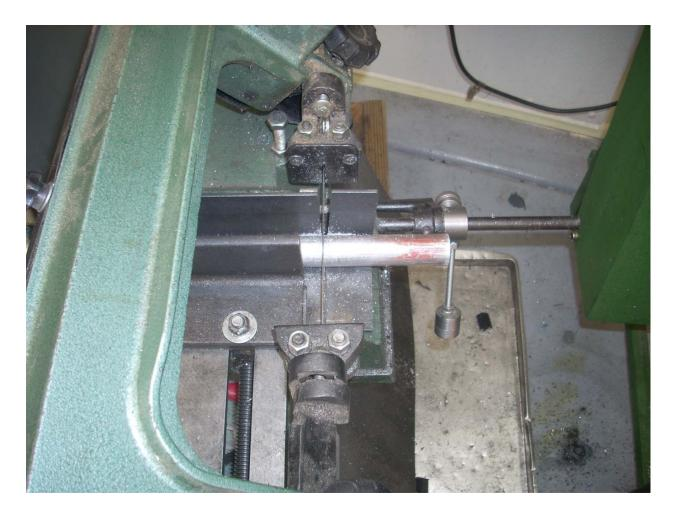
My first step was to cut off about 4" of 1" diameter 6061 aluminum. Then it was chucked into my lathe.
