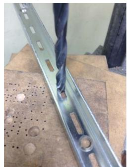
It can be done with a twist drill but often the drill snatches, bends the area around the slot, and flings the workpiece in some random direction.
