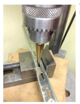
The smallest step drill has a point that fits down in the slot. That lets me center the drill.
