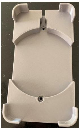
I printed the holder out of PLA in draft mode with 30% fill. If it distorts due to the Arizona heat, I will reprint it with PETG.
