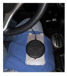
My solution was to 3D print a holder that bolts onto a beanbag. A recess in the holder is a close fit to a magnetic charger disk.
