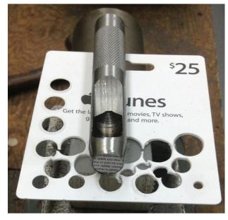
A sharp tap with the hammer on the end of the hollow punch and I have my washer blank. My backing block is soft enough to not damage the cutting edge of the punch yet firm enough to support the plastic sheet. You can see the blank stuck in the end of the punch.
