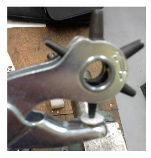
I found it easier to center the revolving hole punch on the blank than to punch the center hole first and then try to align the hollow punch. Try it both ways to see which works best for you.
