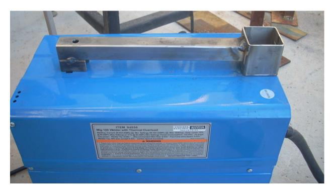
My welder weights around 45 pounds. It came with this flimsy plastic handle. Making things worse, it was a reconditioned unit and the handle was damaged. So it was just a matter of time before it would fail. Rather than tempt fate, I decided to replace it. The plastic handle was the extreme of inadequate. My new handle is close to the extreme of overkill.
