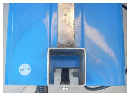
The handle was fitted such that it will not come off. This weld between handle and vertical tube would have to be ground off if I ever do need to remove the handle.
