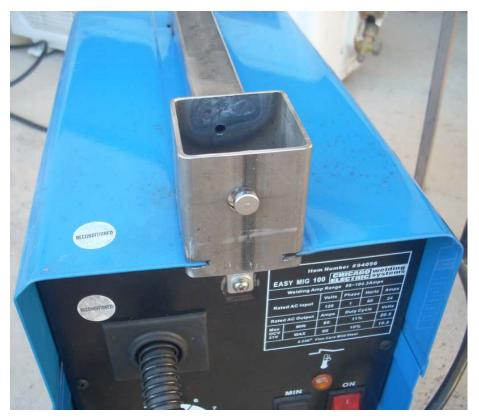
I did not measure anything in the fabricating of this handle. It was all cut to fit. I used my bandsaw to shape the various parts.
