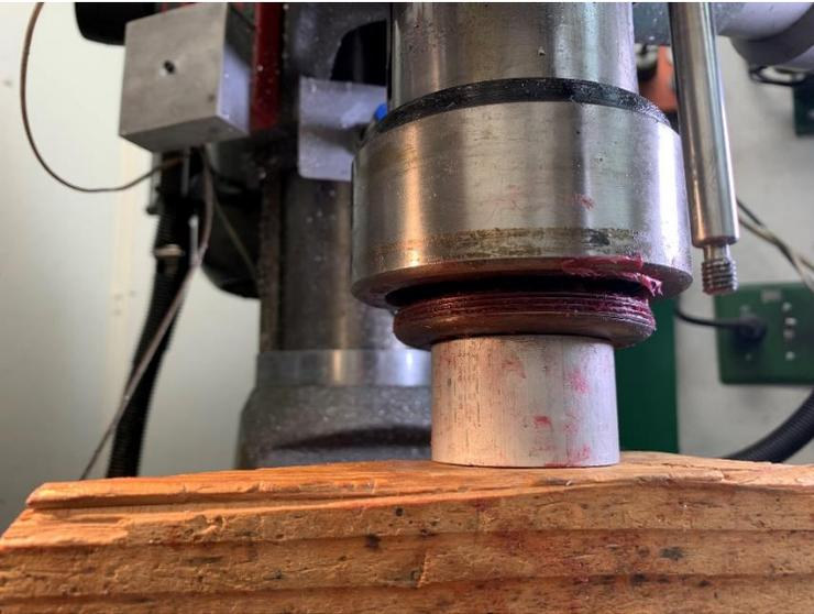
After the usual false starts, I selected a short length of aluminum thick-walled tubing. It cleared the spindle while supporting the cup.
