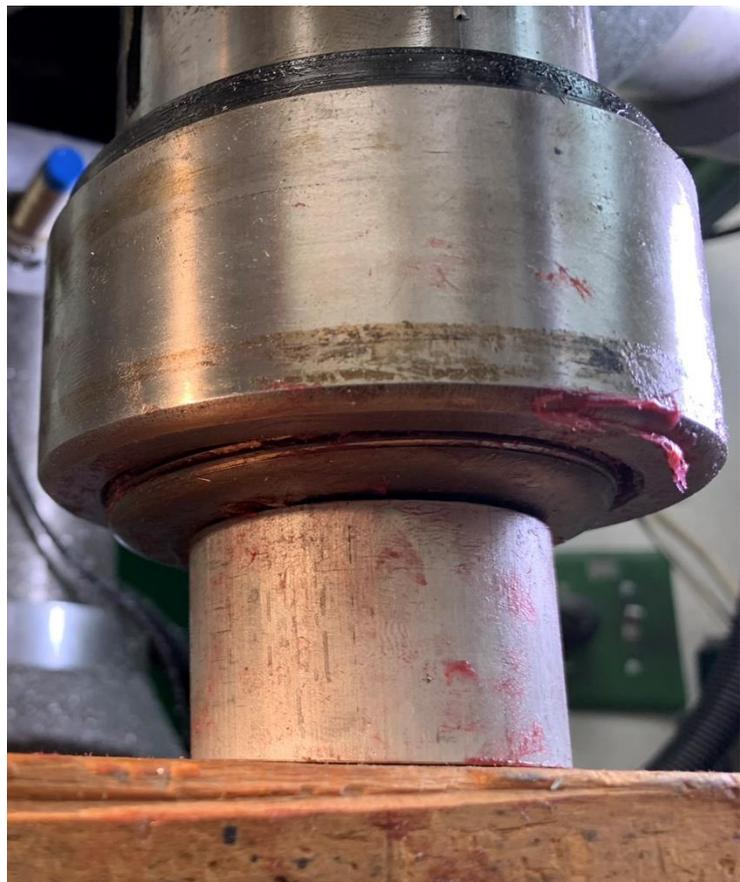
Then I slowly fed the Z axis down until the cup was inside the end of the spindle. The trick was to get the threads close enough that I only had to turn the cup to engage the threads.
