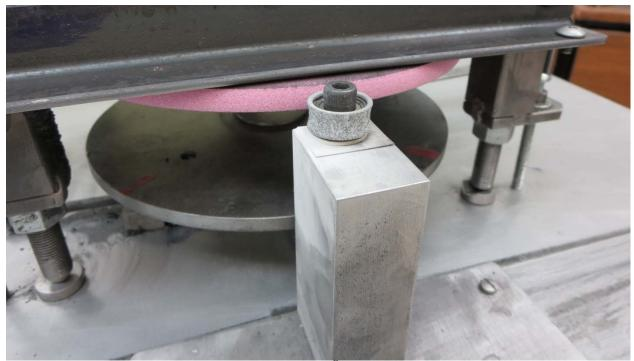
The grinding wheel comes from Blackstone<sup>®</sup> who makes commercial figure skate sharpening machines. This wheel is 100 grit and specifically designed for figure skate sharpening. I dress the wheel with a diamond coated bobbin also sold by Blackstone. This is how I form the 7/16" radius of hollow.
