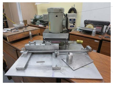
The motor is a <sup>1</sup>/<sub>2</sub> HP Baldor<sup>®</sup>, sealed 3 phase motor with a fan on top. Thanks to Brian Lamb for helping me select the correct HP. Thanks to Dealers Industrial Equipment for helping me select the exact motor and speed control.
