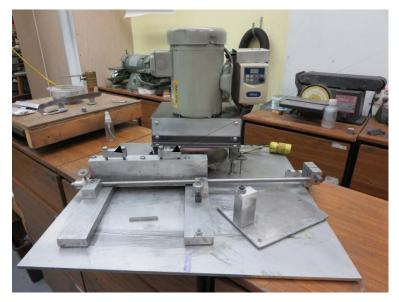
The skate is secured to the carriage with two clamps. This is necessary because often the skate blade has a slight bow in it due to less than perfect mounting. The clamps force the blade flat so the sharpening is uniform. When the clamps are removed, the bowed blade will have a congruent sharpening which is essential for proper operation.
