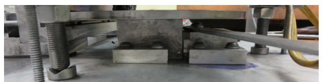
The follower wheel is supported by the follower wheel support block. Behind it is the depth of grind (DOG) support block. Both are captured by dovetails and can be individually locked.
