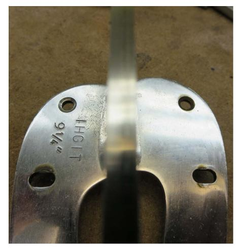
Here is a close up of the ground blade. I have a pair of worn out blades for all testing. New blades cost over \$400. You can imaging the tension in the room when I started to sharpen the good blades!
