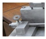
It is essential that the grinding wheel not touch the front pick so that gap is set next. A stop clamped to the far end of the guide bar prevents the user from sliding the pick into the grinding wheel.
