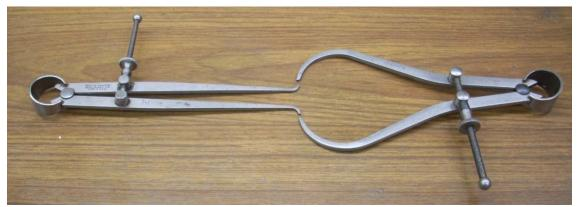
But this time we will use our outside caliper to measure the inside caliper.
