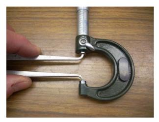
We again start by setting our mic to 0.9000" and then adjust the inside caliper for a sliding fit with no deflection.
