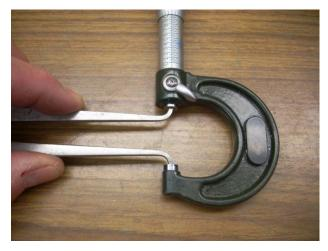
The reading you get on the mic reflects the sum of a number of errors. There was error transferring the mic's opening to the inside caliper. Then we have the error transferring the inside caliper's opening to the outside caliper. This was followed by the error of using the inside caliper to read the outside caliper. And finally, we have the error associated with using the mic to read the inside
