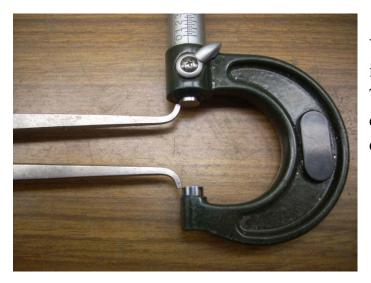
You should be able to start with the inside caliper just off of the mic. Then slide it in and feel a slight drag but no compression of the caliper<sup>3</sup>.
