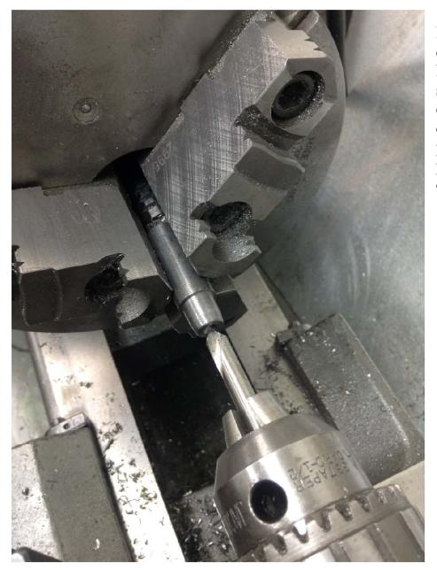
In preparation for drilling the .201" hole, I used a spotting drill to cut a cone shaped depression. This prevents the drill point from moving off center.
