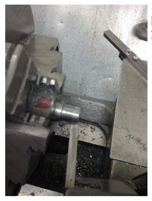
I then used my parting tool to cut a bevel on the end. It is done by eye because accuracy is not important here.
