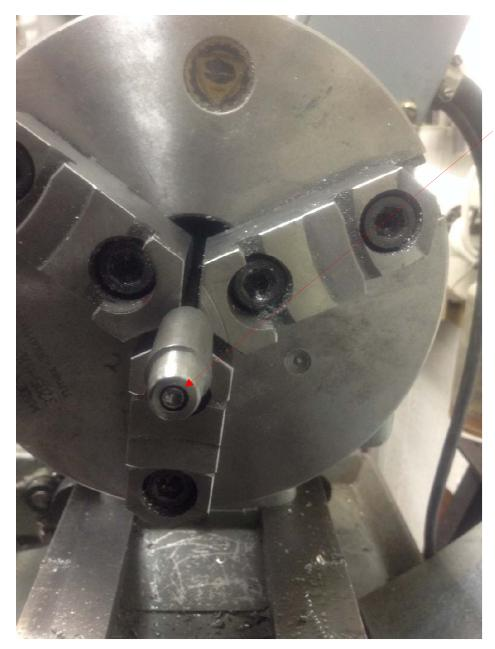
The sleeve is threaded onto the rod. You can now see the cone shaped hole in the end of the rod.
