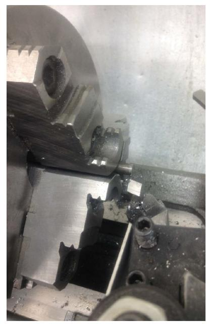
The workpiece was turned end for end with about  $\frac{1}{2}$ " sticking out. I then faced the end and deburred it. Leaving it in the chuck, I measured its overall length. Then I fed in the apron and cut the length to 1.5"  $\pm 0.01$ ".
