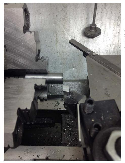
After sawing off a 1.55" length of <sup>1</sup>/<sub>2</sub>" diameter CRS, I faced the end using my Diamond Tool Holder and deburred with a file.
