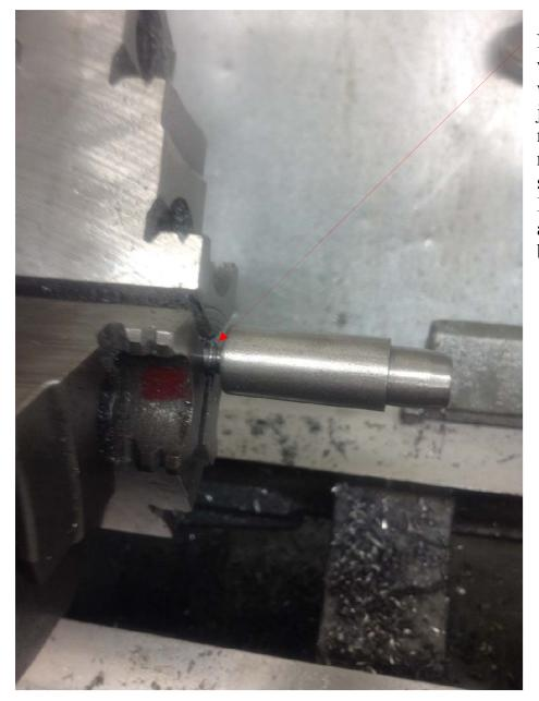
Note that the sleeve was not in contact with the face of the jaws. The next machining step required maximum support for the rod so I loosed the chuck and slid the assembly back.
