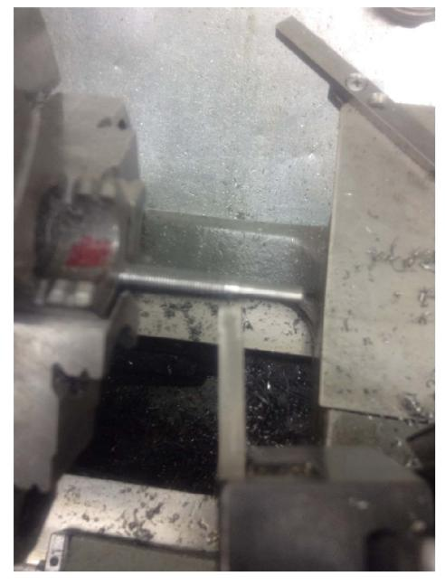
Then the rod was reposition to have 1.8" exposed. This was a minor error because I needed to cut a bevel to allow for the partial thread. This is really excessive overhang when using a parting tool. But I went slow and was not taking much metal so got away with it.
