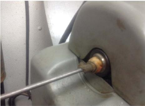
The rod was about 2 feet long so must pass through the hollow spindle of my lathe. A piece of fabric was stuffed around the rod to prevent excessive flopping about.
