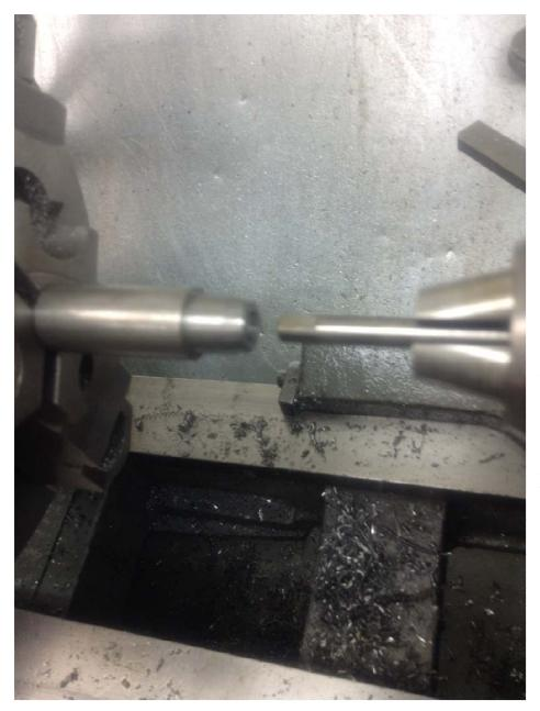
I mounted a piece of broken tap into my drill chuck. The end of this tool was ground flat. It is about 0.18" across.
